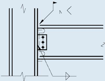
For joints in special moment frames, inelastic deformations in beams and column panel zones are more reliably attained with ASTM A992 wide-flange shapes.
