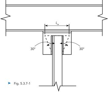
5.3.7. How can adequate flexibility be maintained in double-angle simple shear connections subjected to combined shear and tension load?
