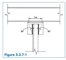
the end of a connection resisting tension or compression, such as that from a brace-togusset-plate connection or similar fitting. As illustrated in Figure 5.3.7-1 for a WT hanger connection, the effective length for the Whitmore section  $L_w$  is determined using a spread-out angle of 30° along both sides of the connection, beginning at the start of the connection. It is applicable to both welded and bolted connections.
