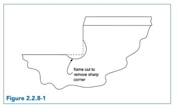
solution is to flame-cut additional material at the corner to provide a smooth transition as illustrated in Figure 2.2.8-1. Note that the sides of the cope need not meet the radius transition tangentially. Any notches that occur at re-entrant corners should be repaired as indicated in 2.2.7.
