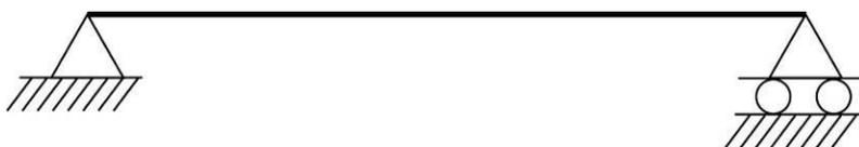
**Figure 3.14.1-1. Simple-span beam with statically determinate boundary conditions.**
