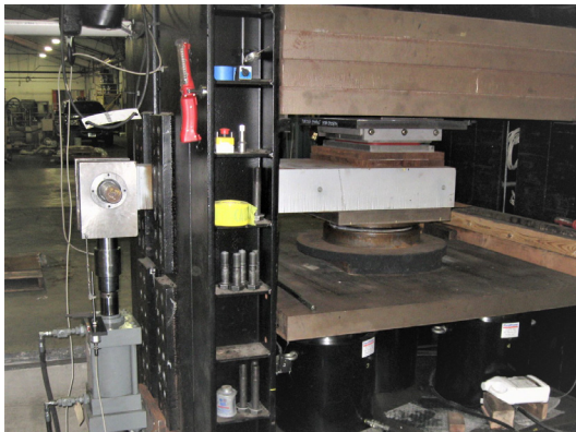
Figure 3.5-1. Long-Term Deterioration Test (Cyclic Rotation Test Frame)
