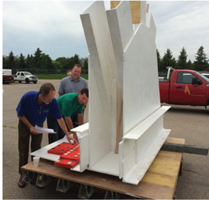
Figure A3.5.4-1—Plywood mockup of retrofitted Winona Bridge through-truss joint.
