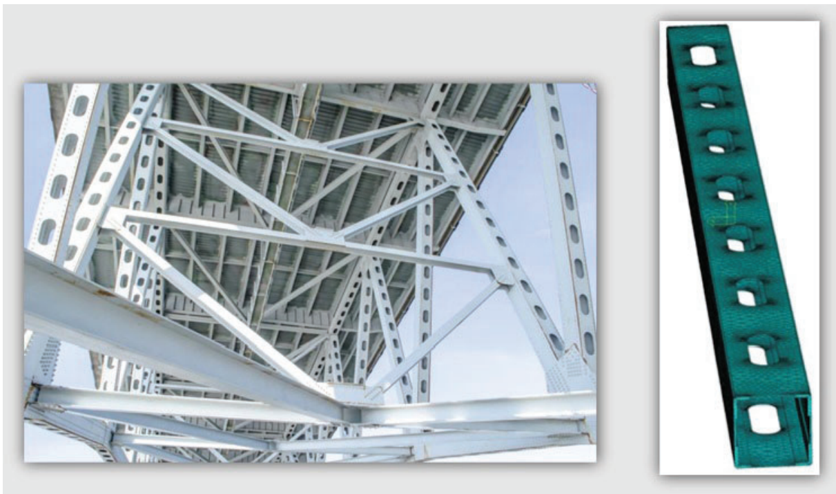
Figure A3.3.3-1—High-resolution three-dimensional solid model of a single truss member with cut-outs.
