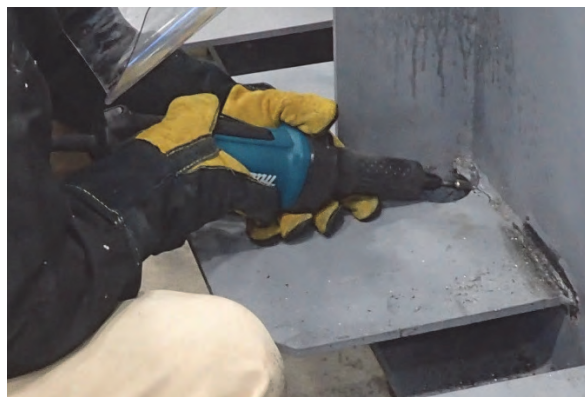
Figure 3-10. Typical Angle Grinder with Flap Wheel Figure 3-11. Typical Die Grinder with Burr Bit
