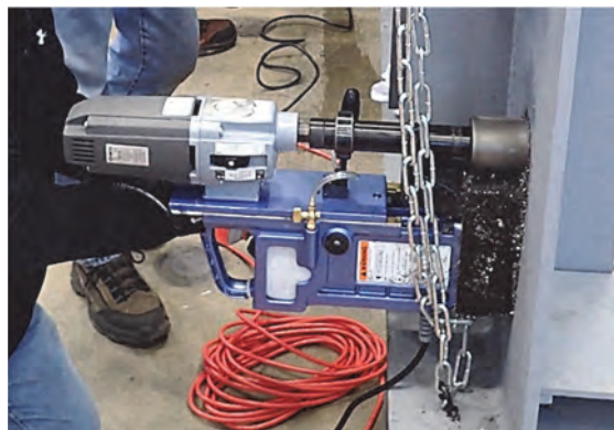
Figure 3-1. (Left) Example of Magnetic-Based Drill, (Right) Annular Cutter Used for Hole Drilling
