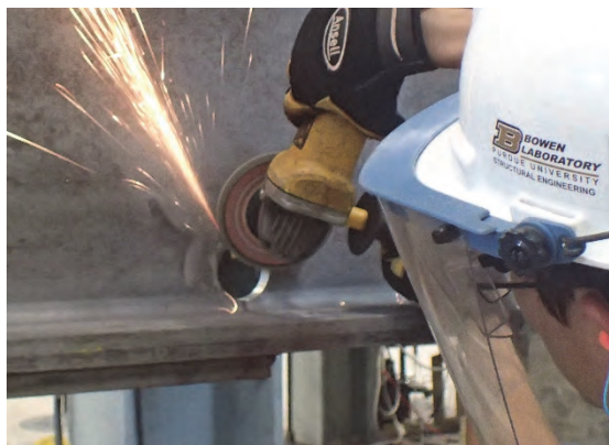
Figure 3-10. Typical Angle Grinder with Flap Wheel Figure 3-11. Typical Die Grinder with Burr Bit
