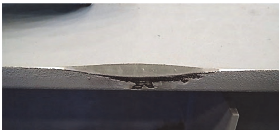
Figure 4-17. Example of Edge Flaw Removed with 5:1 Fairing Ratio, Shown Prior to Repainting
