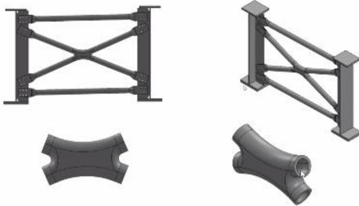
out to be bolted to the transverse stiffener plate. Angles could also be used instead of tubular sections. Karl mentioned how University of Texas at Austin had looked at steel castings for cross-frames and Carlos was aware of this work and that tubular sections can be more expensive to fabricate than angles and WT members. Ronnie agreed with
