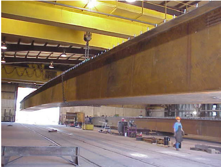
Figure 3- A Box Girder in the Shop
