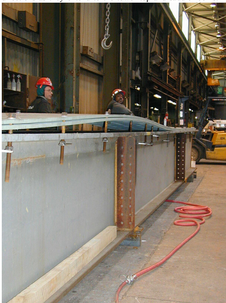
Figure 4. Steel erector's shop test of reinforcing plate tightening procedure, before performing the operation on the bridge.
