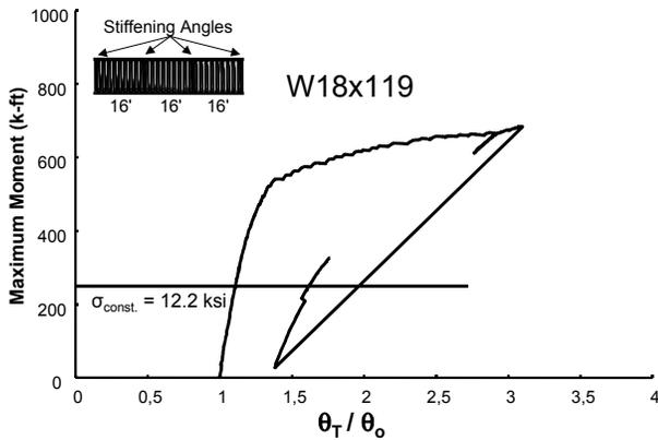
**Figure 10: Test results for W18x119 girders with PMDF for bracing.**
