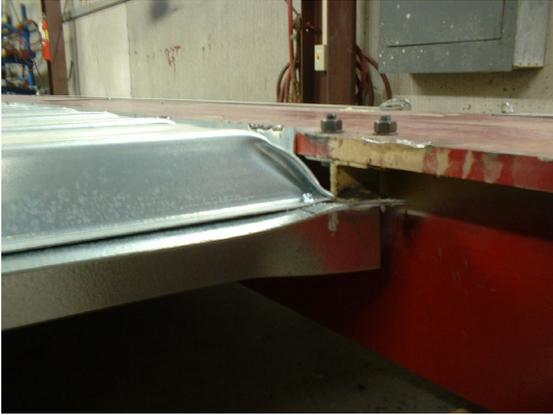
**Figure 5: Stiffening angle detail at failure.**
