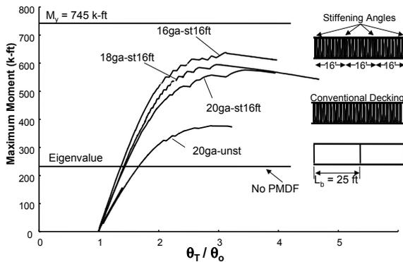
**Figure 9: Test results for twin girder system with PMDF bracing.**
