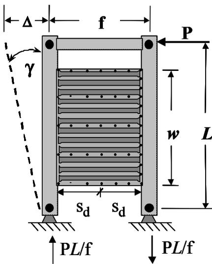
Figure 2: Shear frame for measuring PMDF stiffness and strength.
