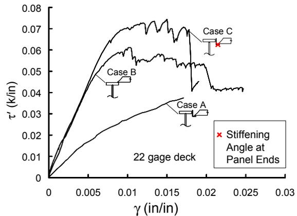
**Figure 7: Effective shear Stress versus shear strain.**
