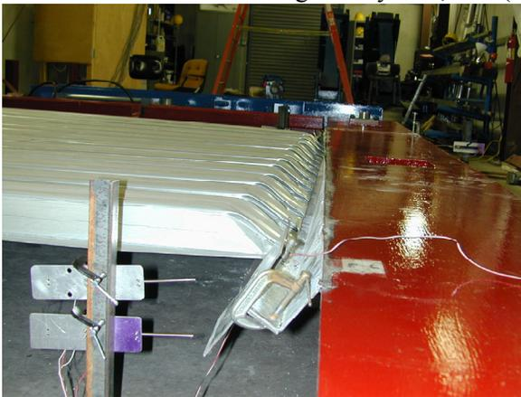
**Figure 3: Rotation of support angle using conventional connection detail.**
