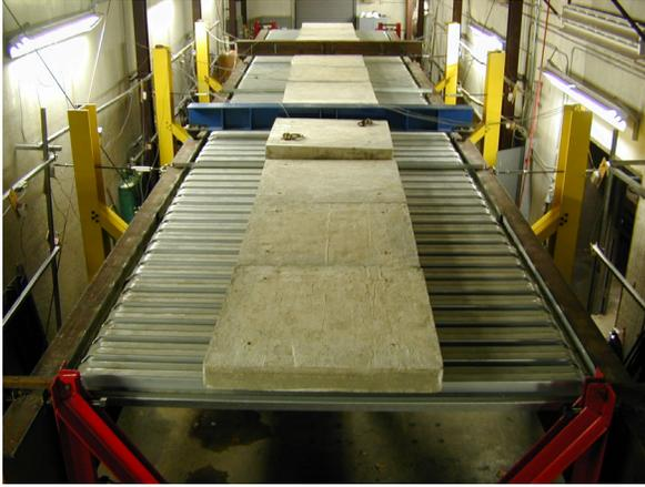
**Figure 8: Twin girder system with PMDF bracing.**
