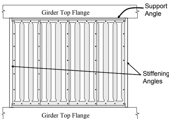
**Figure 4: Plan view of stiffening angle layout.**
