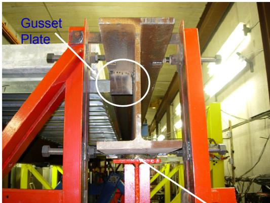
**Figure 6: Alternate Stiffening Angle Detail.**
