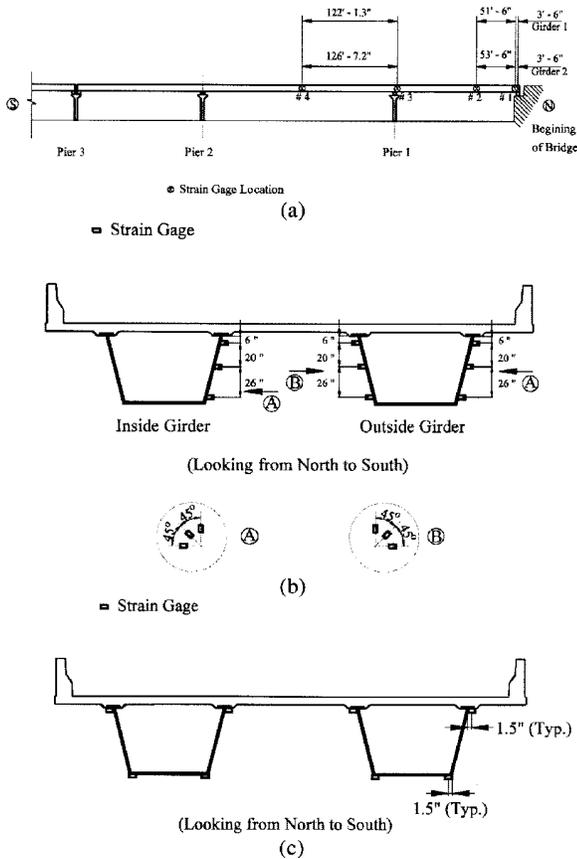
**Figure 3: Strain Gage Locations, (a) Longitudinal Direction, (b) Transverse Direction at Section #1, (c) Transverse Direction at Sections # 2 to 4.**
