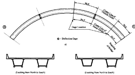
Figure 5: Locations of Vertical Deflection Gages, (a) plan, (b) Cross-section of Side Span, (c) Cross-section of Center spans.
