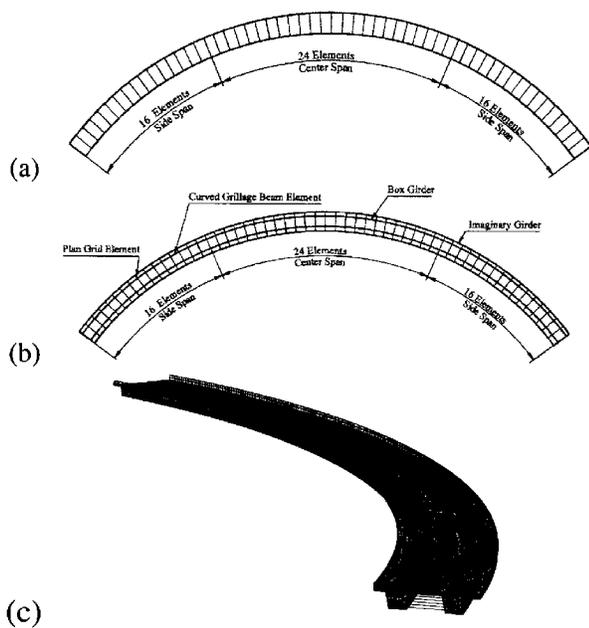
Figure 9: Analytical Model, (a) Plane Grid, (b) Curved Grillage Beam, (c) Shell-plate
