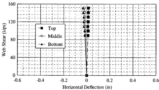
Figure 12: Web Shear – Lateral Deflection Curves of Outside Web of Outside Girder
