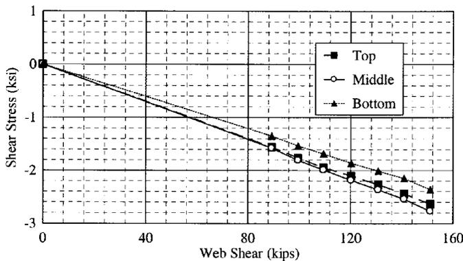
Figure 11: Web Shear-Shear Stress Curves of Outside Web of Outside Girder
