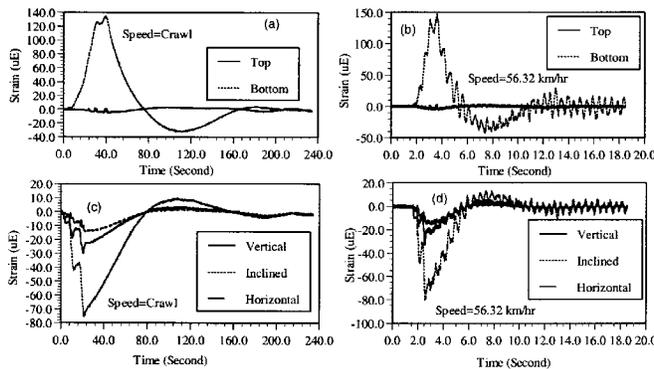
**Figure 14: Typical Time Histories, (a) Strain in Outside Web of Outside Girder at Section 2 (crawl), (b) Strain in Outside Web of Outside Girder at Section 2 (35 mph), (c) Strain at Middle of Outside Web at Section 1(crawl), (d) Strain at Middle of Outside Web at Section 1 (35 mph)**
