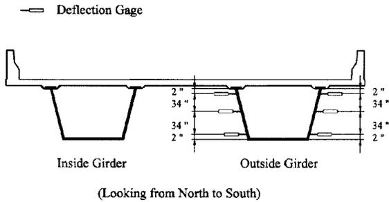
Figure 4: LVDT Deflection Gages at Section #1.
