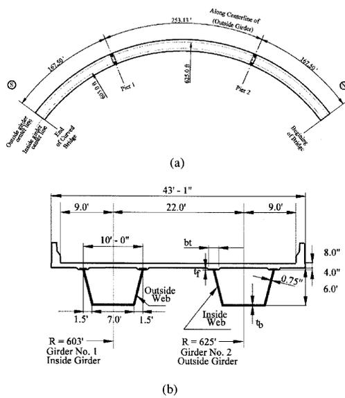
**Figure 2: Veteran's Memorial Curved Bridge, (a) Bridge Plan, (b) Typical Cross-Section**
