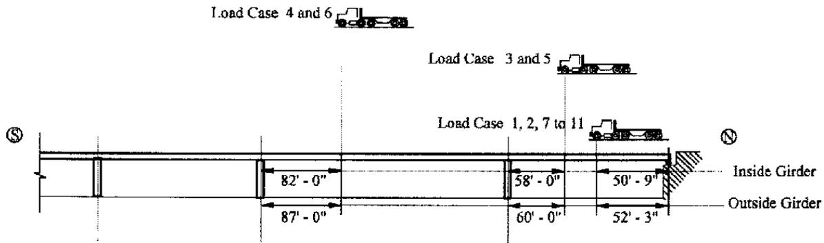
Figure 7: Truck Longitudinal Locations
