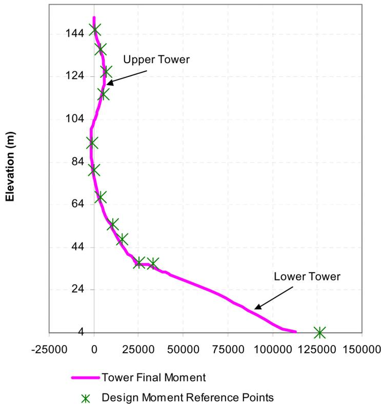
Figure 6: Tower Moment Diagram (KN-m/10)
