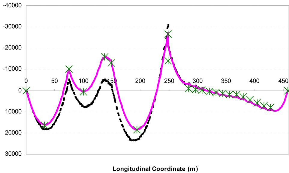
Figure 5: Final Box Girder Moment Diagram (KN-m/10)
