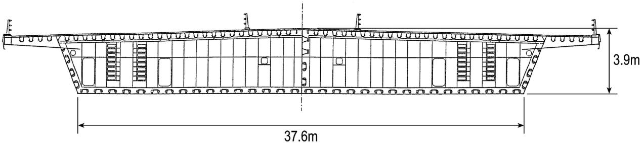
Figure 2: Steel Orthotropic Box Girder
