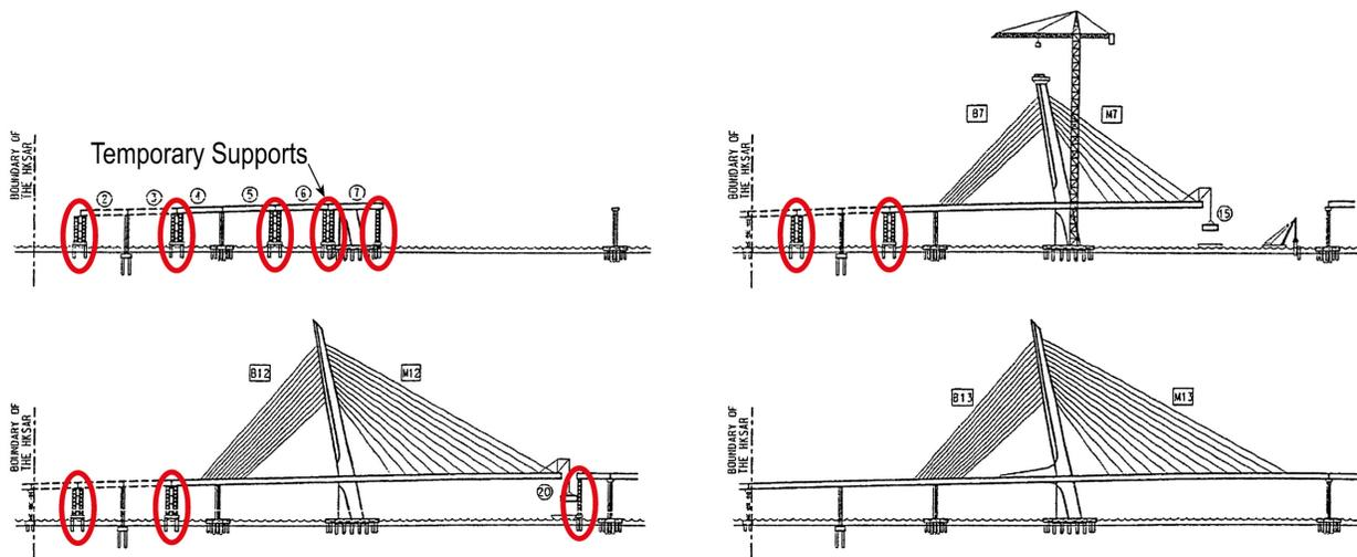
*Figure 3: Erection of back span in half-length units, simply supported on permanent piers and temporary towers. After they are connected and made continuous, the temporary support towers are removed; Erection of typical segments concurrently with the tower; Erection of last bridge segment (closure); Bridge completion.*
