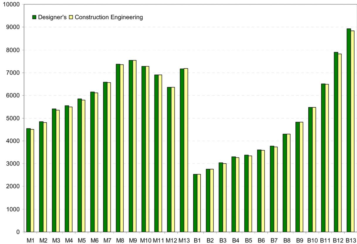
Figure 7: Final Cable Forces (KN)
