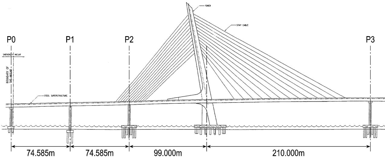
Figure 1: Cable-Stayed Bridge Layout
