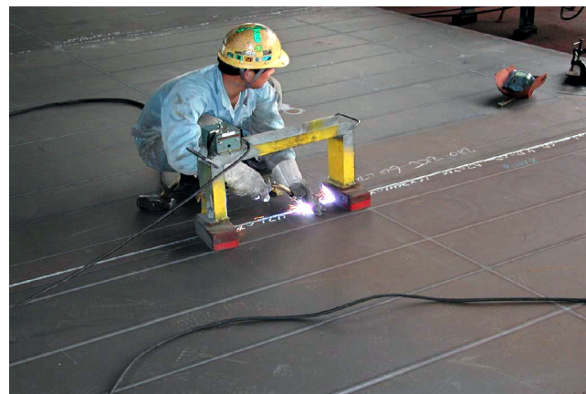
Through out-of-position welding achieves high quality, welding is generally more cost effective when accomplished in the flat position.
