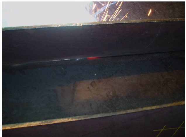
Melt through should not be confused with blow through; however, occurrence of more than occasional melt through should be addressed.
