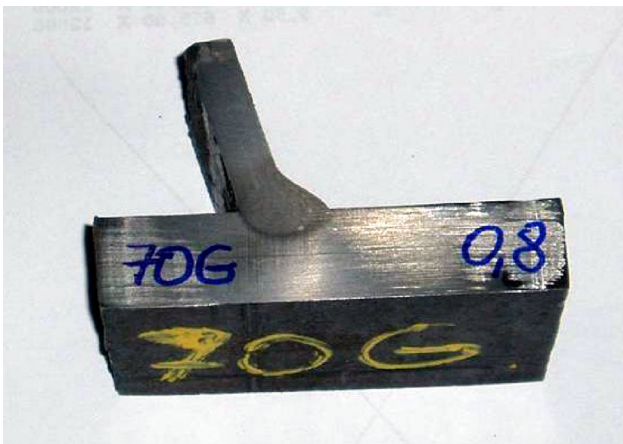
Remelting 90% of rib to deck tack welds results in retempering of the remaining 10%.
