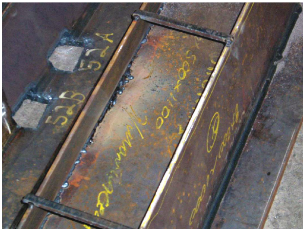
Melt through should not be confused with blow through; however, occurrence of more than occasional melt through should be addressed.
