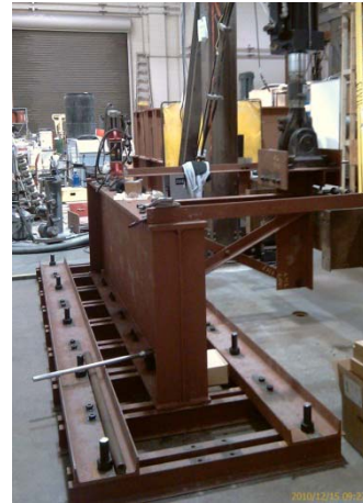
Figure 2. View of fascia side of girder specimen
