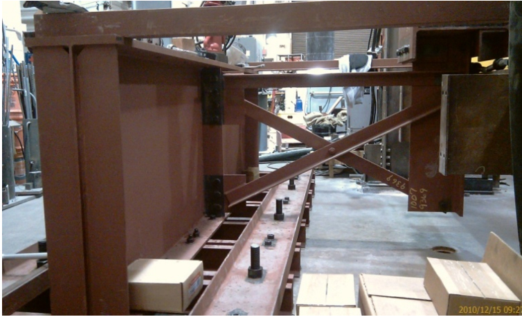
Figure 1. View of of girder specimen
