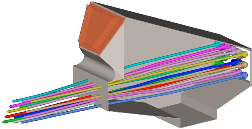
Figure 12 – Post-Tensioning Tendons through Knuckle
