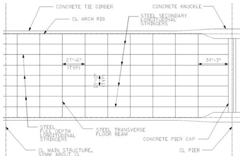
Figure 5 – Floor System Framing Plan
