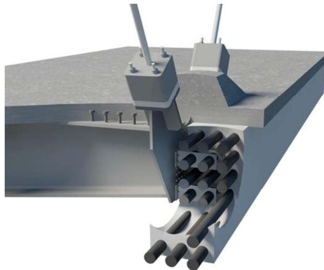
Figure 11 – Post-Tensioned Concrete Tie Girder
