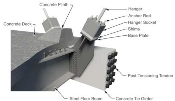
Figure 14 – Lower Hanger Connection
