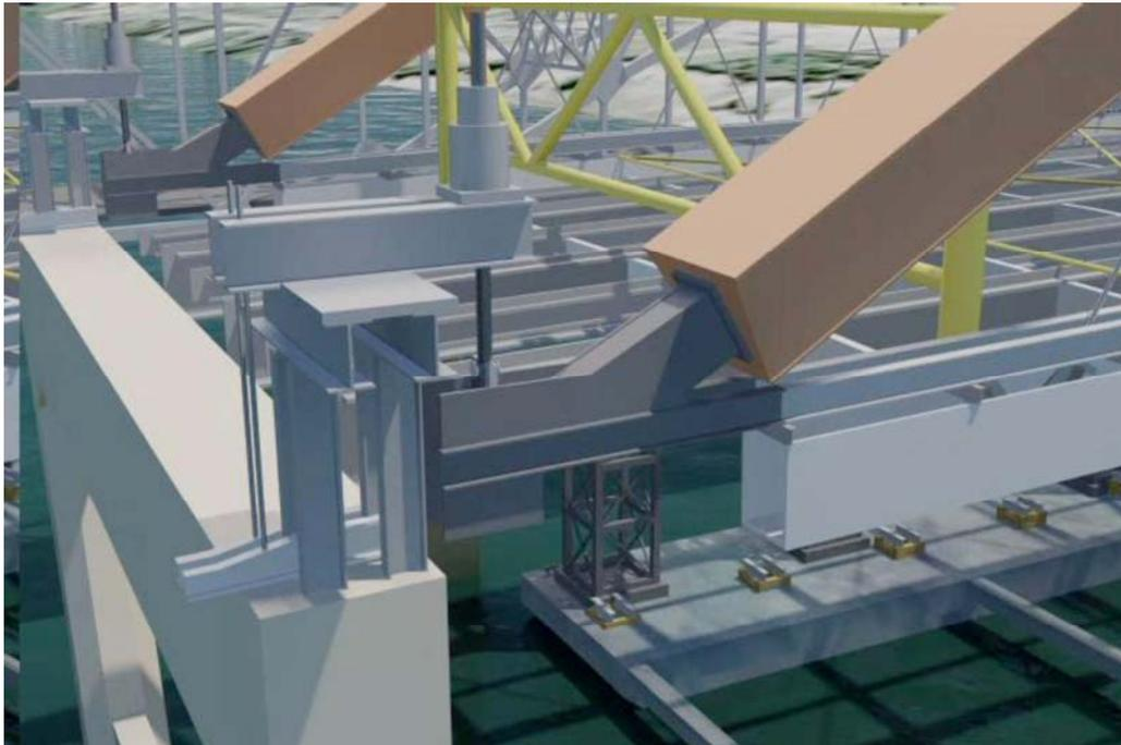
Figure 17 –Lifting Frame and Strand Jacks
