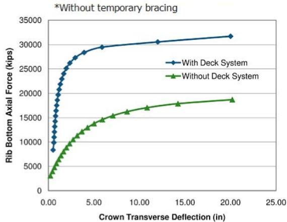
Figure 9 – Buckling Analysis Results
