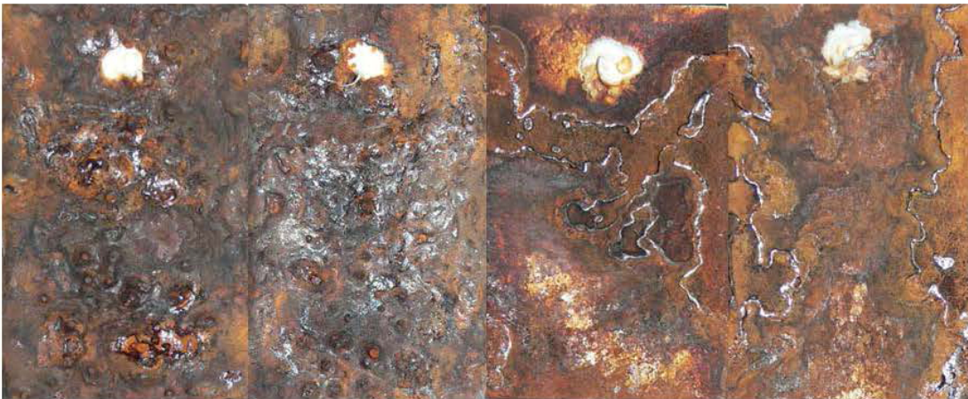
(c) Sealed container with water reservoir and salt spray 2/week.
