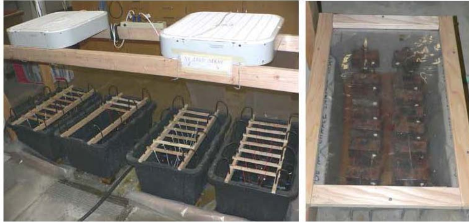
Figure 6. Test setup. Photo on the left shows the samples hanging in basins (two left) for fresh water spraying and the fan on the top for drying and similarly the two right basins for fresh water and salt water plus drying. Photo on the right shows the salt spray-only samples inside the covered container.
