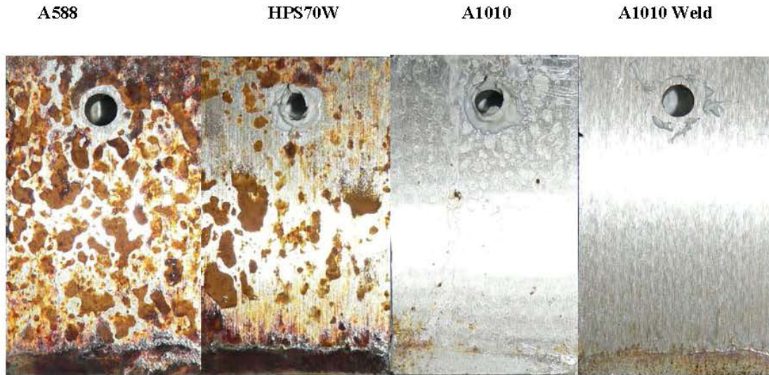
(a) Fresh water exposure 4/day.
