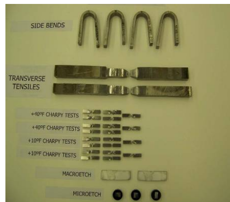
(b) test samples of welding process
