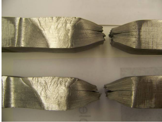
Figure 5. Transverse Tensile Test, no lamellar indication was observed.
