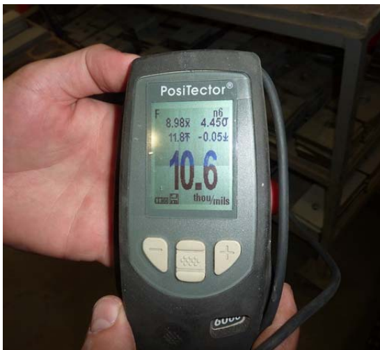
Figure 3: Coating thickness measurement using a PosiTector Magnetic Gage
