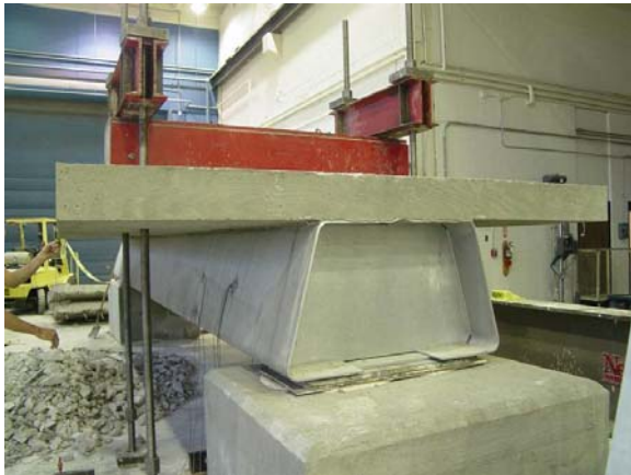
Figure 11. Test E2 – Load Configuration
