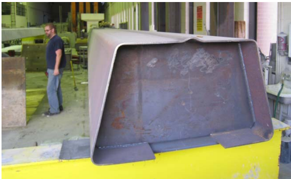
Figure 3. 46 ft. Long Folded Plate Girder
