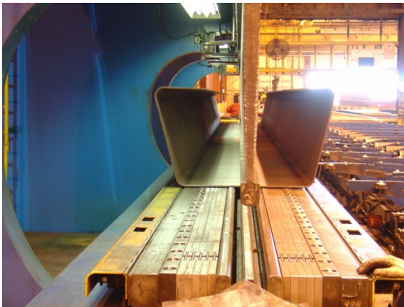
Figure 1. Fabrication of folded plate girder using a press break machine
