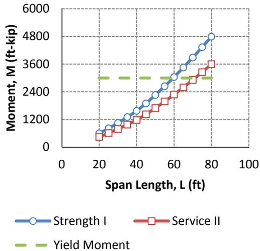
Figure 4 Design Evaluations for a Press-Brake Tub Girder (96" × 1/2" Standard Mill Plate)
