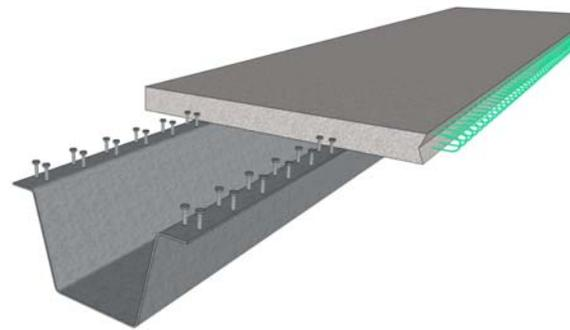
Figure 1 Conceptual Composite Press-Brake Tub Girder
