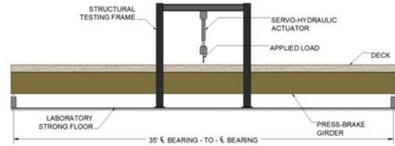
Figure 5 Typical Test Setup
