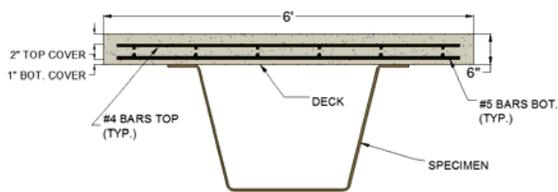
Figure 8 Deck Design for Composite Girder Specimen
