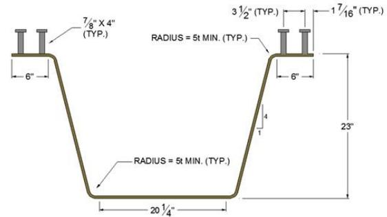
Figure 6 Testing Specimen Dimensions
