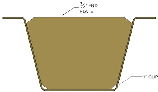
Figure 7 Tub Girder Bearing Plate
