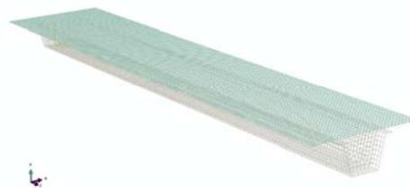
Figure 10 Finite Element Model of Composite Press-Brake Tub Girder Specimen
