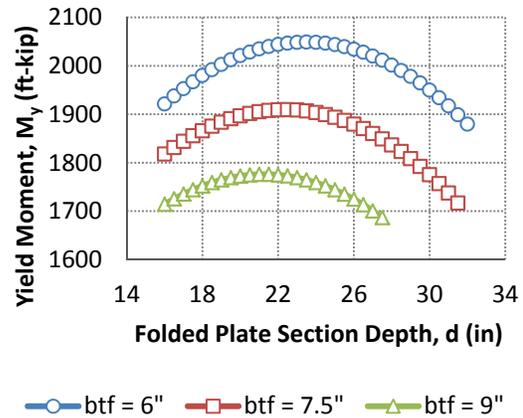
Figure 3 Preliminary Design Comparisons for an 84" × 7/16" Standard Mill Plate
