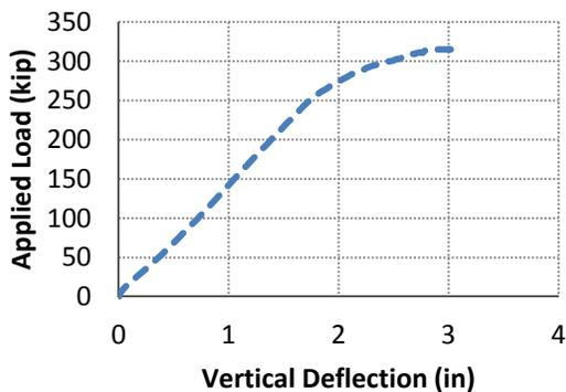
Figure 9 Load-Deflection Response of Specimen One
