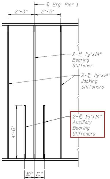
**Figure 7:** Auxiliary Bearing Stiffeners and Future Jacking Stiffeners at Pier 1 (shown) and Pier 4 (similar)
