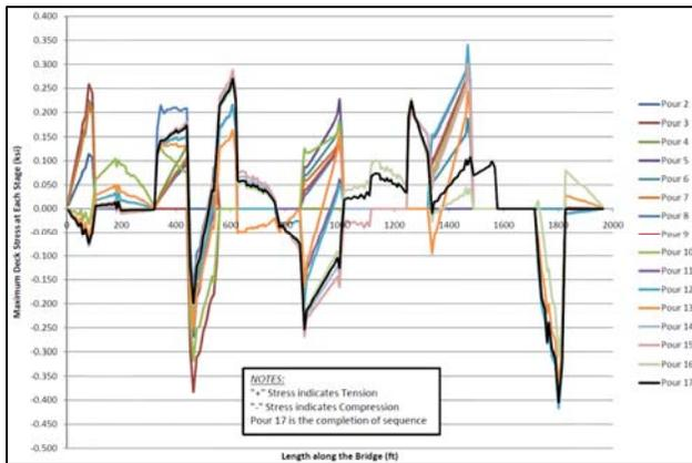
**Figure 11:** Maximum Predicted Deck Stress for Each Stage of the Deck Placement Sequence
