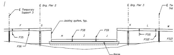
**Figure 12:** Center Span Lift of Girder Segments
