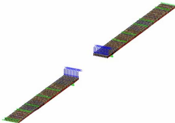
**Figure 13:** 3D Analysis Model for Conceptual Erection Sequence, Center Span Segment Strand Jack Lift
