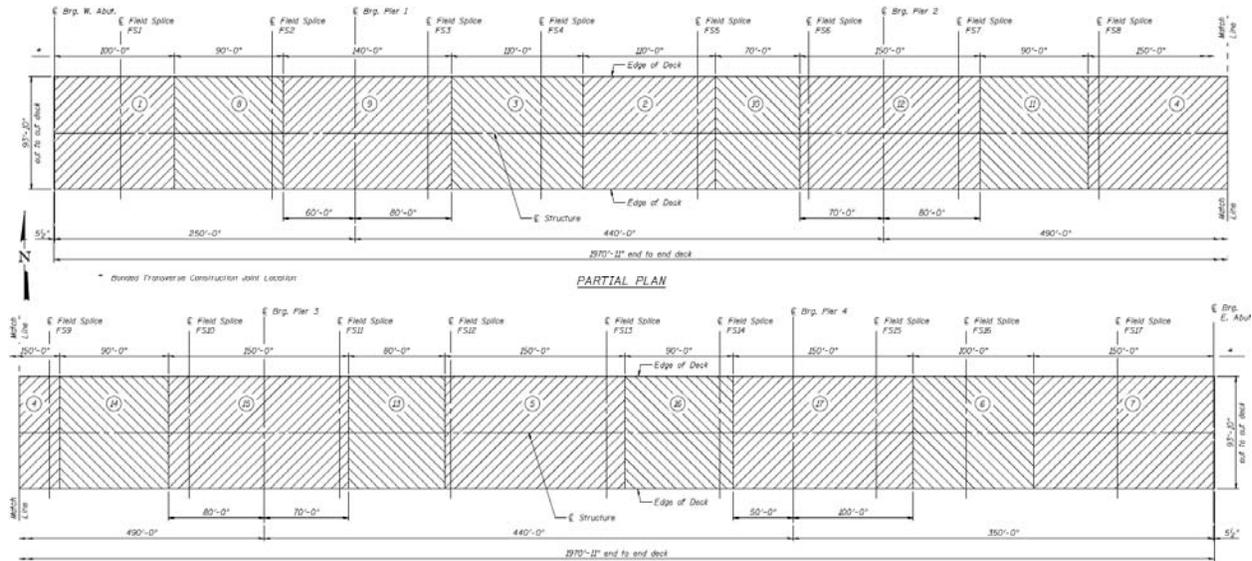
**Figure 10:** Plan View of Deck Placement Sequence
