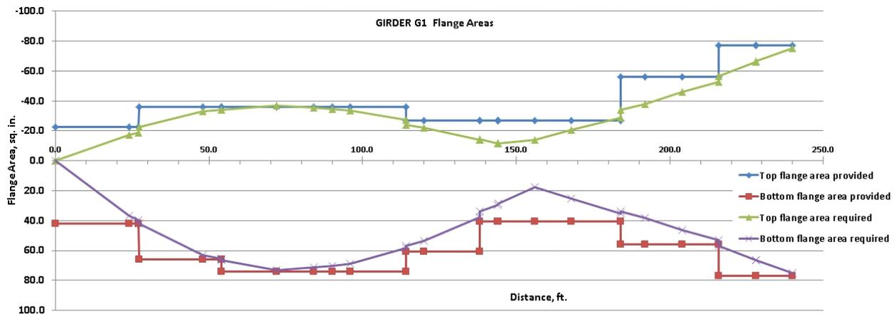
Figure 4. Girder G1, Required and Provided Flange Areas along the Half-Girder
