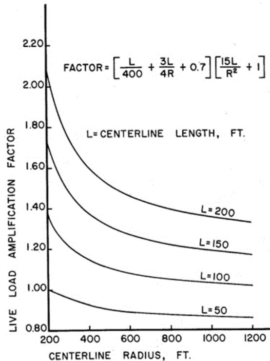
Figure 6. Amplification Factor for Live Load Bending Moment in Longest Curved Girder (5)
