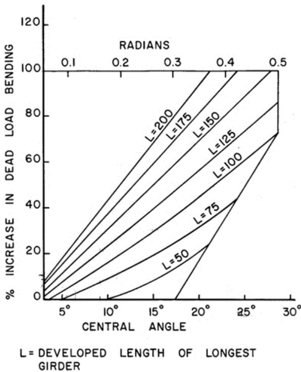
Figure 5. Percent Increase in Dead Load Bending Moment in Longest Curved Girder (5)
