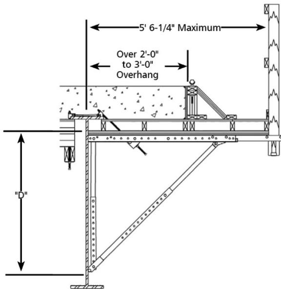
Figure 3. Typical Overhang Form Bracket
