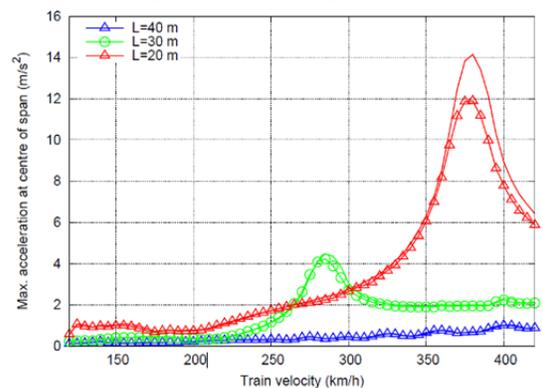
Fig. 6: Midspan vertical accelerations due to a given moving load train configuration on a simply supported bridge, for different span lengths and different train speeds. Note that maximum admissible values are usually between 2 and 4 m/s<sup>2</sup>. From Goicolea (5).
