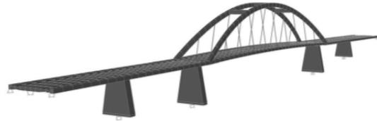
Fig. 10: 3D Frame-member structural model used for static pre-dimensioning.
