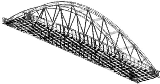
Fig. 11: 3D view of the final design, with tubular diagonal members.
