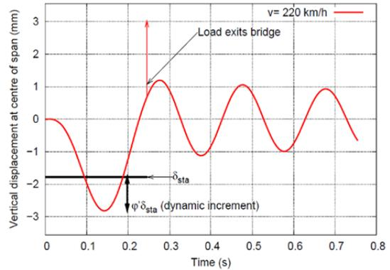
Fig. 4: Midspan vertical deflections due to a moving load on a simply supported bridge, compared with the static deformation ( $\delta_{sta}$ ). Note that the deck continues moving after load has gone out.
