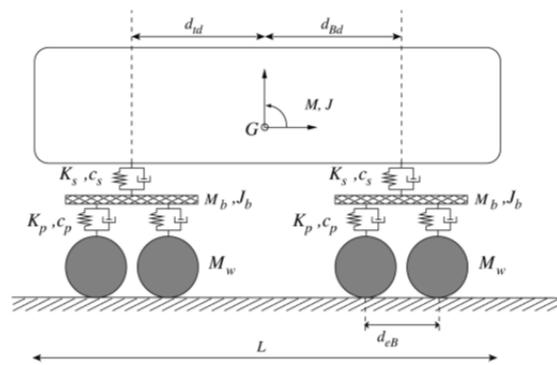
Fig. 5: Complete model of a train wagon used for dynamic analysis. Mass spatial
