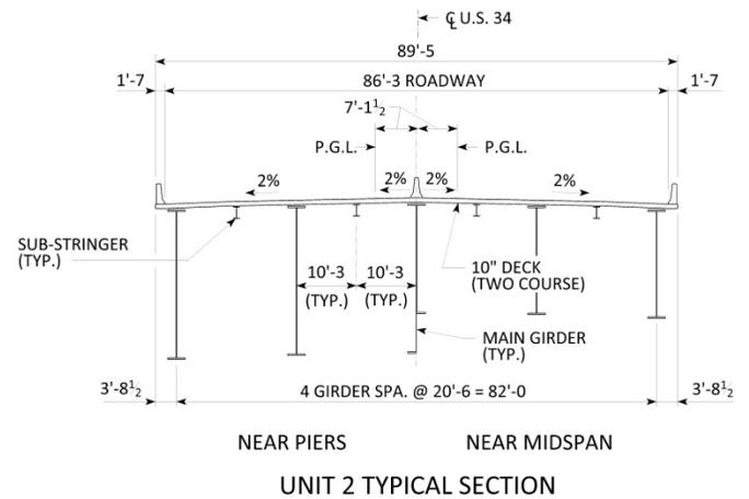
Figure 1: Typical Section - Main River Unit
