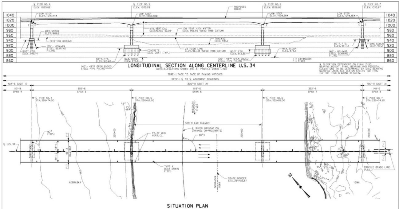
Figure 2: Plan & Elevation – Main River Unit
