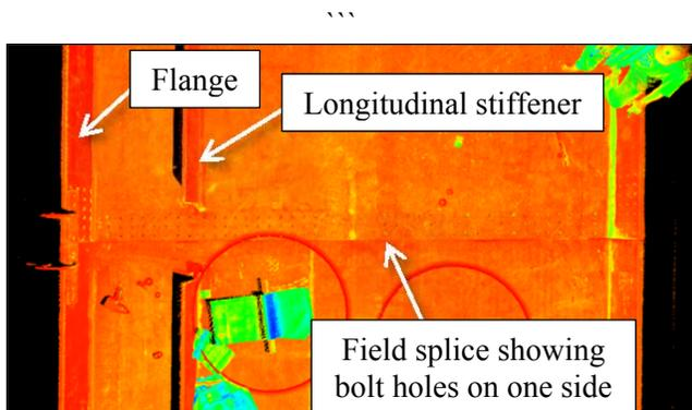
**Figure 3:** Laser Scan of Field Splice
