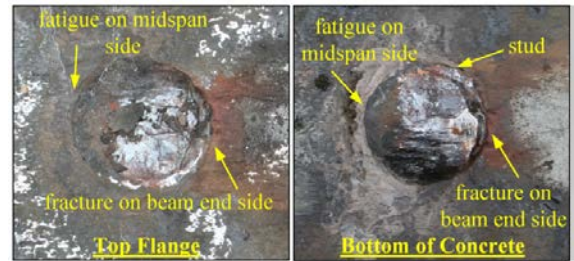
Figure 7. Photo of shear stud fracture surfaces
