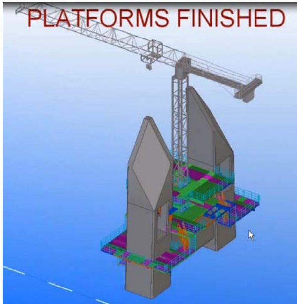
Figure 2 – From 3D model for planning tower top platform installation.
