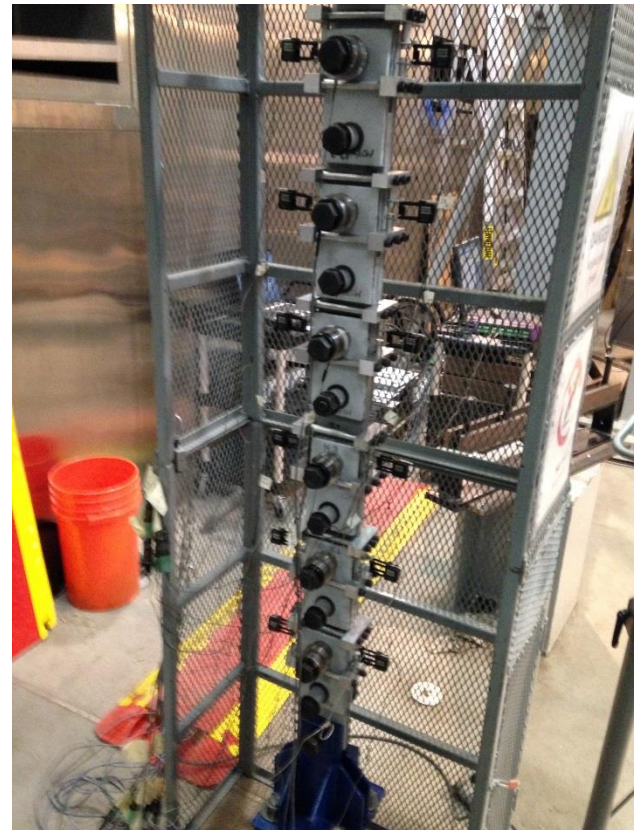
Figure 4: Creep test set-up
