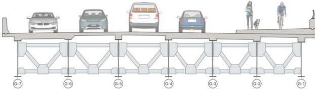
Figure 4. Ultimate Bridge Typical Section.
