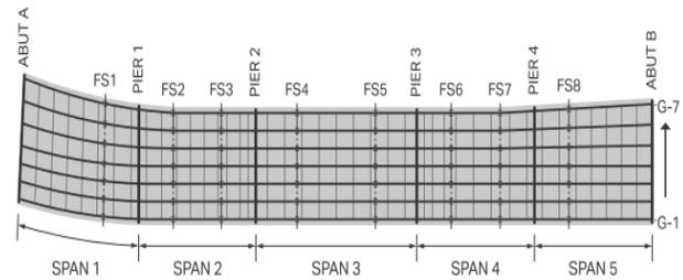
Figure 5. Framing Plan.
