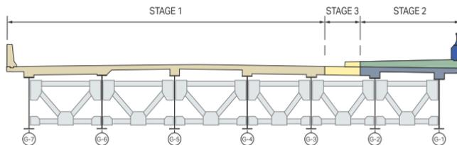
Figure 7. Proposed Sequence of Construction.
