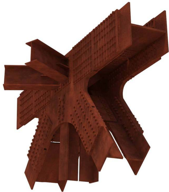
Figure 12 - Rendering of Top Chord Connection
