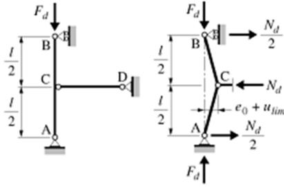
Figure 2. Nattere et al., discrete point column bracing (reproduced)
