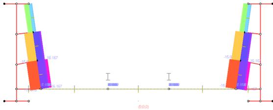
Figure 9. LARSA Knee Brace flange force showing both tension and compression
