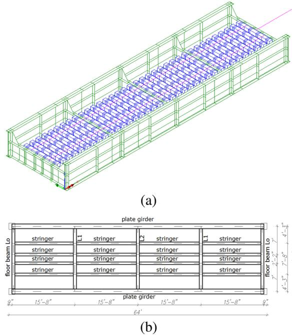
Figure 5. LUSAS TPG Model for floorbeam-stringer system (a) overall model, and (b) framing plan layout
