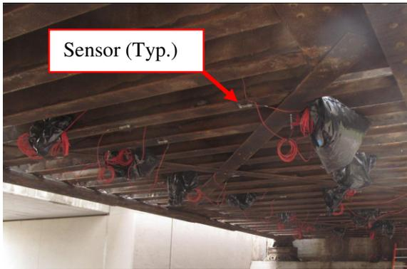
Figure 16. Strain gages applied to TPG (showing underside of bridge)
