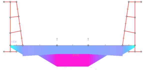
Figure 14. Moment in floorbeam for associated knee braces in compression (grey) and tension (purple/pink) demonstrating qualitative controlling moment condition
