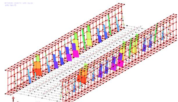
Figure 11. Knee Brace flange forces for E80 Cooper loading
