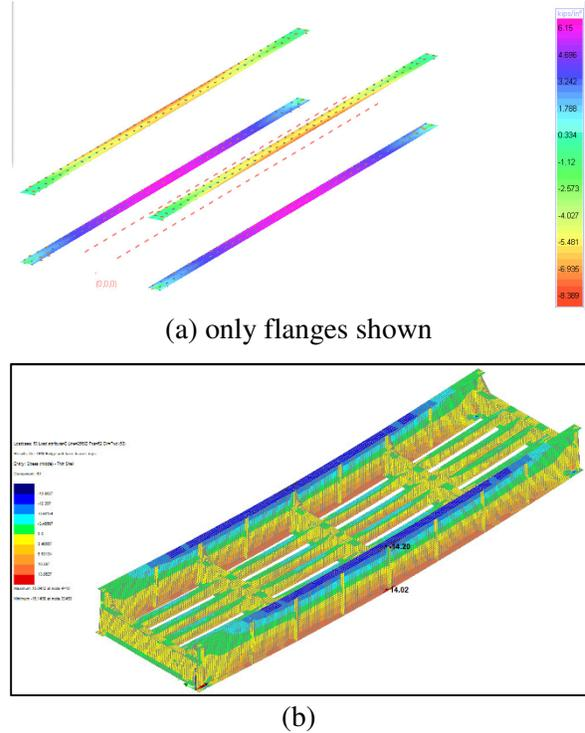
Figure 8. TPG stress profile showing (a) 6.2kip of in compression flange for the LARSA Model and (b) 14.2kip of compression flange for the LUSAS Model.
