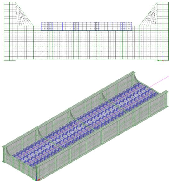
Figure 6. Finite element mesh for TPG floorbeam-stringer system
