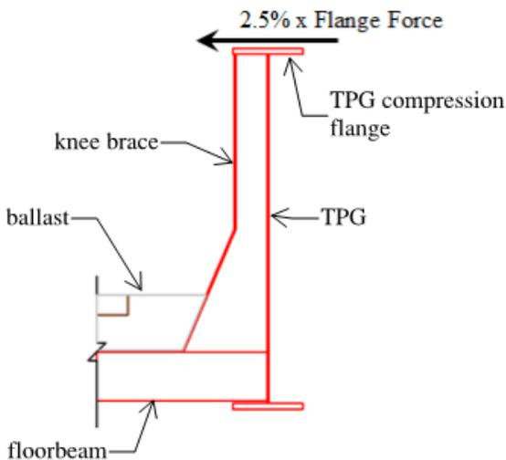
Figure 1. TPG section showing knee brace notional load
