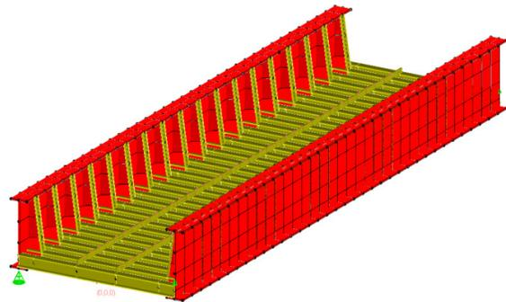
Figure 4. LARSA TPG Model for floorbeam only system
