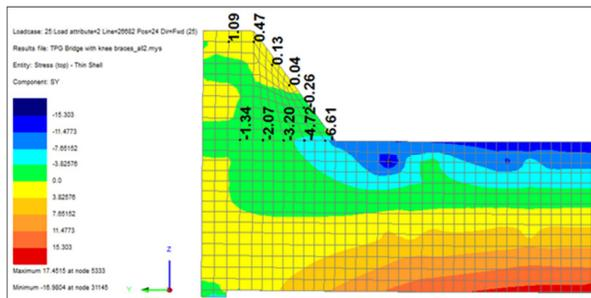
Figure 10. LUSAS Knee Brace plate stresses showing both tension and compression
