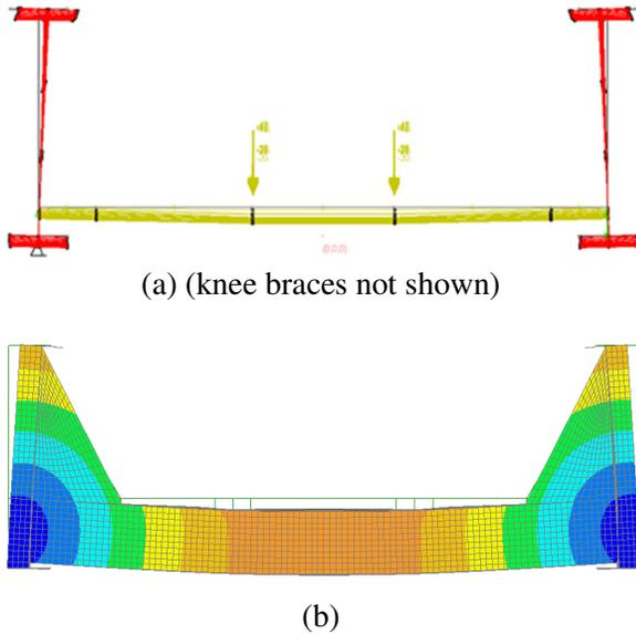
Figure 7. TPG deflected shapes and torsional rotation for (a) LARSA Model and (b) LUSAS Model
