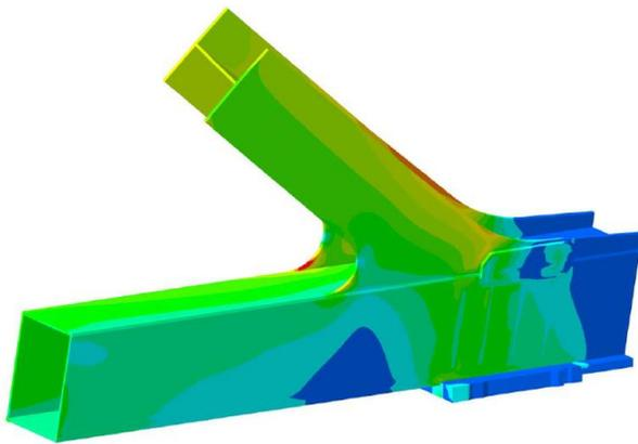
**Figure 8: Knuckle Vertical Stress**
