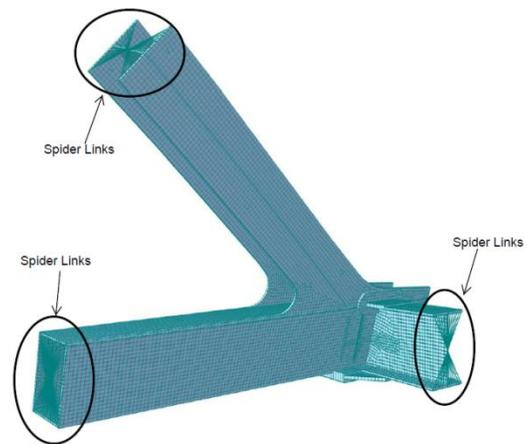
**Figure 7: Finite Element Model of Knuckle Region with Spider Link Elements Shown**
