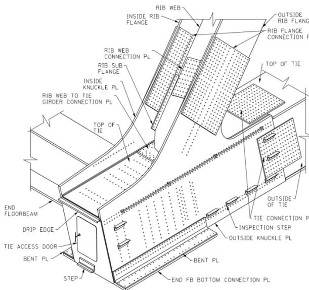
**Figure 6: 3D Isometric View of the Knuckle**
