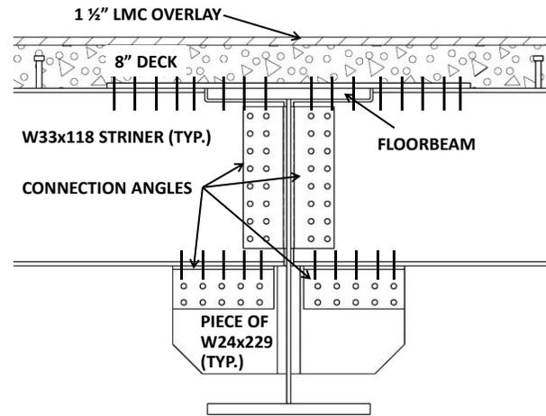
**Figure 5: Integral Floor System**
