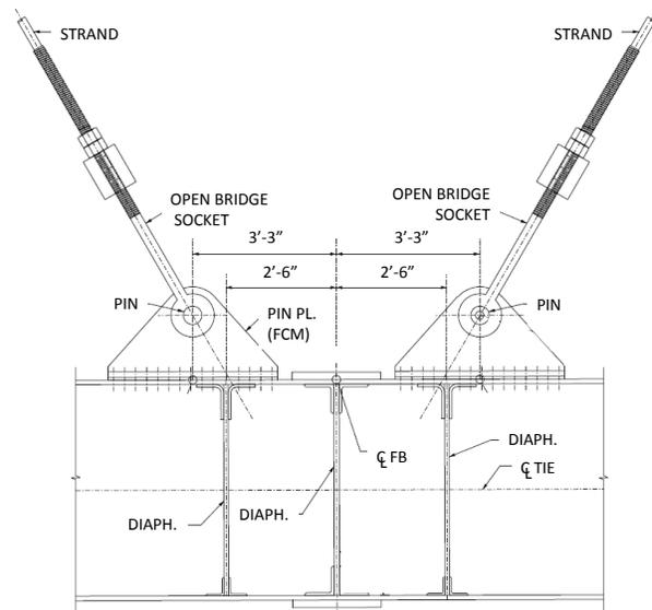
**Figure 11: Hanger Connection at Tie Girder**
