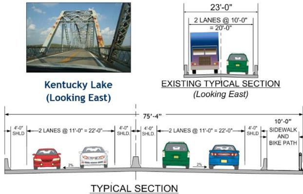
**Figure 3: Kentucky Lake Bridge Typical Section**
