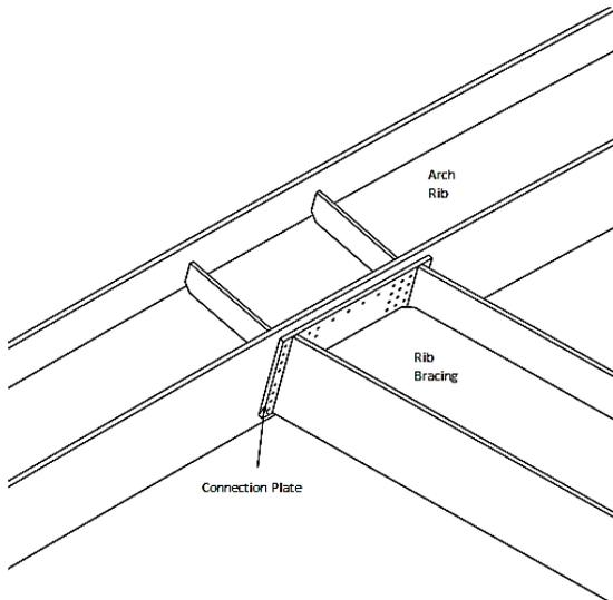
**Figure 10: Isometric View of Rib Bracing Connection**
