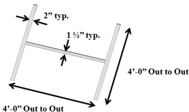
**Figure 9: Typical Section of Arch Rib**
