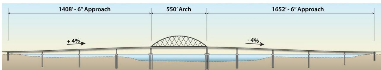
Figure 2: Schematic of KY Lake Bridge Crossing
