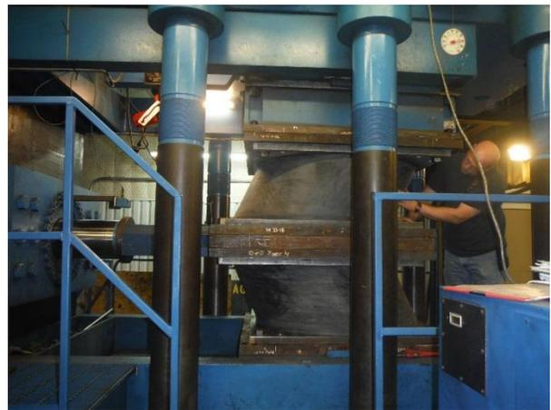
**Figure 12: Seismic Isolation Bearings Verification Test Used on KY Lake**
