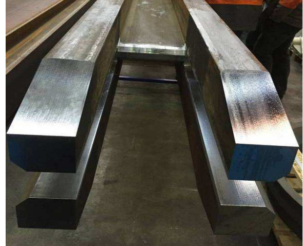
Figure 5: Diagonal of outrigger system with a milling connection detail to fit on a thick gusset plate
