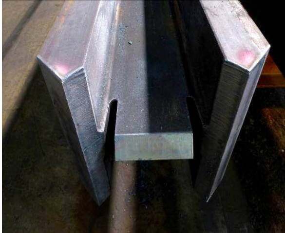
Figure 4: Standard chamfering of Heavy Jumbo shapes by means of flame cutting [1]
