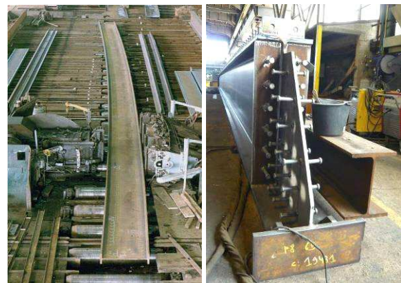
Figure 14: Fabrication of composite bridge girders out of rolled sections – cambering and plate/stud welding [13]
