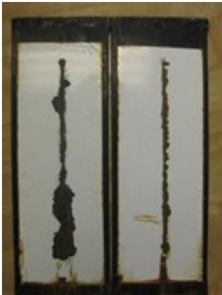
Figure 9: Salt Fog Corrosion Test Results, Polysiloxane and Fluorourethane
