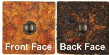
Figure 11: A709 GR50W top plates after 20 cycles of corrosion testing
