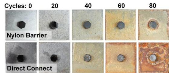
Figure 13: Comparison of direct connect and nylon barrier A709 GR50 HDG top plates
