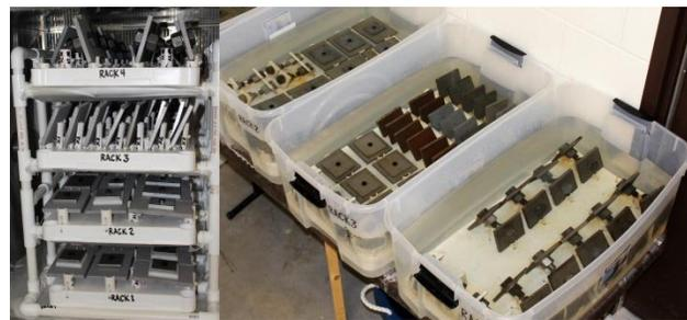
Figure 1: Test specimen configuration in environmental chamber and salt solution
