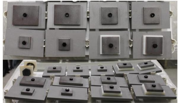
Figure 3: Galvanic corrosion plate assemblies in plastic racks prior to the initiation of testing
