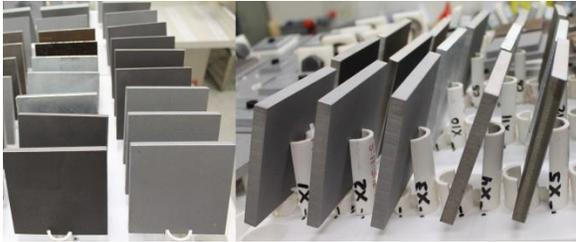
Figure 2: Control plate specimens in plastic racks prior to the initiation of testing
