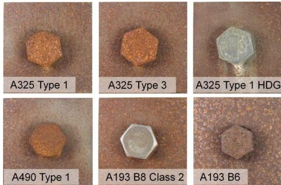
Figure 14: Galvanic corrosion fastener assemblies after 20 cycles of testing.
