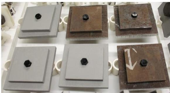
Figure 5: Crevice corrosion fastener assemblies in plastic racks prior to the initiation of testing
