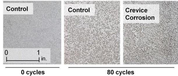
Figure 19: Comparison of A1010 control and crevice corrosion specimens
