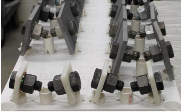
Figure 4: Galvanic corrosion fastener assemblies in plastic racks prior to the initiation of testing
