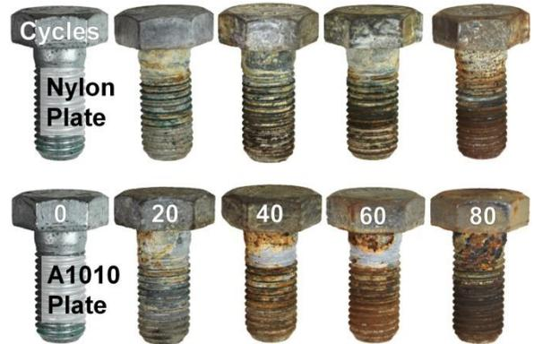
Figure 17: Comparison of A325 Type 1 HDG bolt specimens from nylon and A1010 plate assemblies
