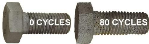
Figure 18: A193 B6 bolt specimens from A1010 plate assembly, showing pitting corrosion
