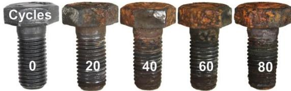
Figure 16: A325 Type 3 bolt specimens from A1010 plate assembly
