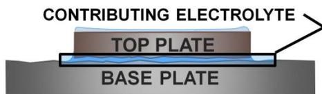
Figure 12: Diagram showing electrolyte permitting galvanic corrosion located primarily between faying surfaces of connected plates
