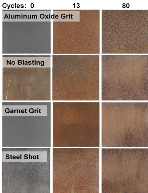
Figure 20: Comparison of A1010 surface preparation plate specimens at early and late stages of testing
