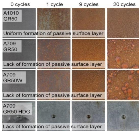
Figure 7: Control plate specimens through 20 testing cycles
