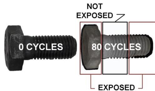
Figure 15: Depiction of relative thickness loss of bolt material based on level of exposure of surface
