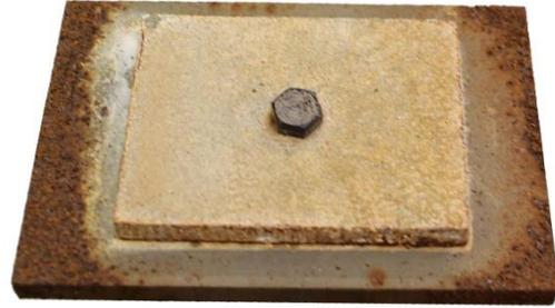
Figure 9: Galvanic protection occurring on A1010 base plate connected to HDG coated A709 top plate
