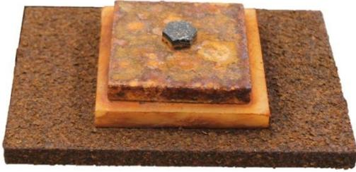
Figure 8: Unstable corrosion occurring on A1010 base plate connected to uncoated A709 top plate
