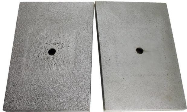
Figure 10: A1010 base plates from direct connect A709 assemblies, GR50 (left) & GR50 HDG (right)
