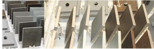
Figure 6: Surface preparation plate specimens in plastic racks prior to the initiation of testing
