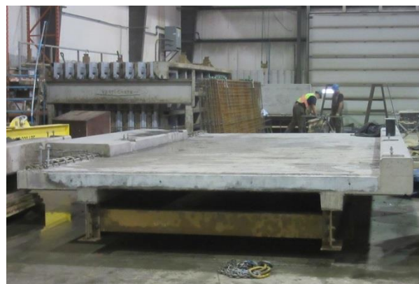
Figure 20 – Precast Sidewalk Unit
