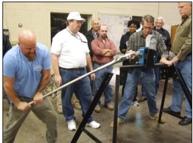
Figure 9. Demonstration of B8-2 bolt acceptance testing.
