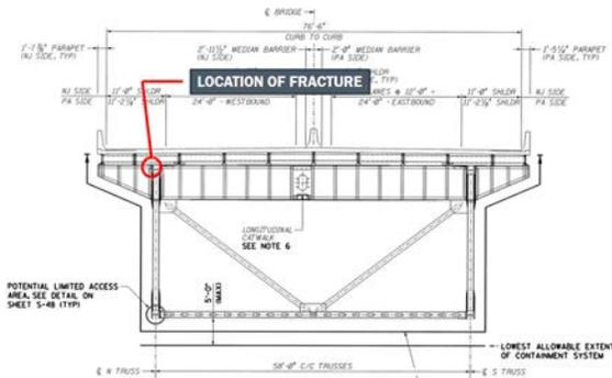
Figure 2 Cross Section of Truss Spans
