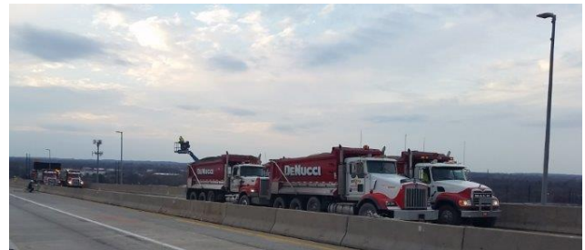
Figure 11: Load Test Trucks in Position
