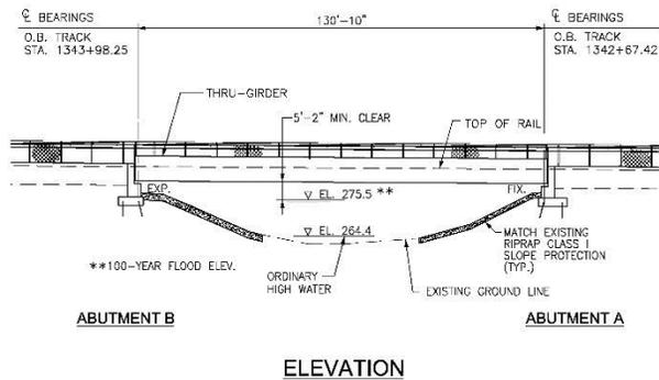
**Figure 8:** Horsepen Run Bridge span configuration.
