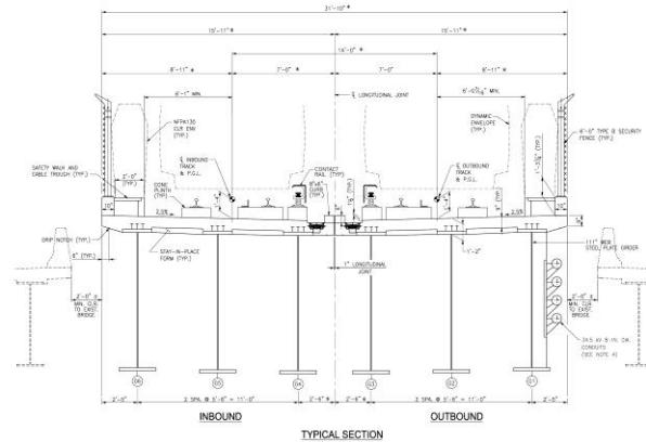
**Figure 14:** Typical section of Broad Run Bridge.
