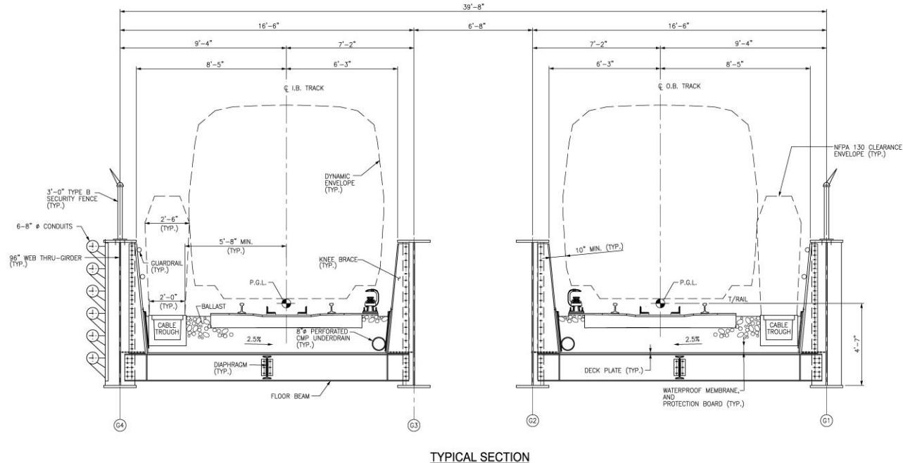
**Figure 9:** Typical section of Horsepen Run Bridge
