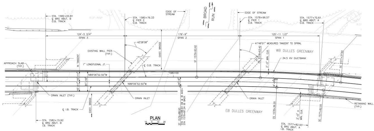
**Figure 13:** Span layout of Broad Run Bridge
