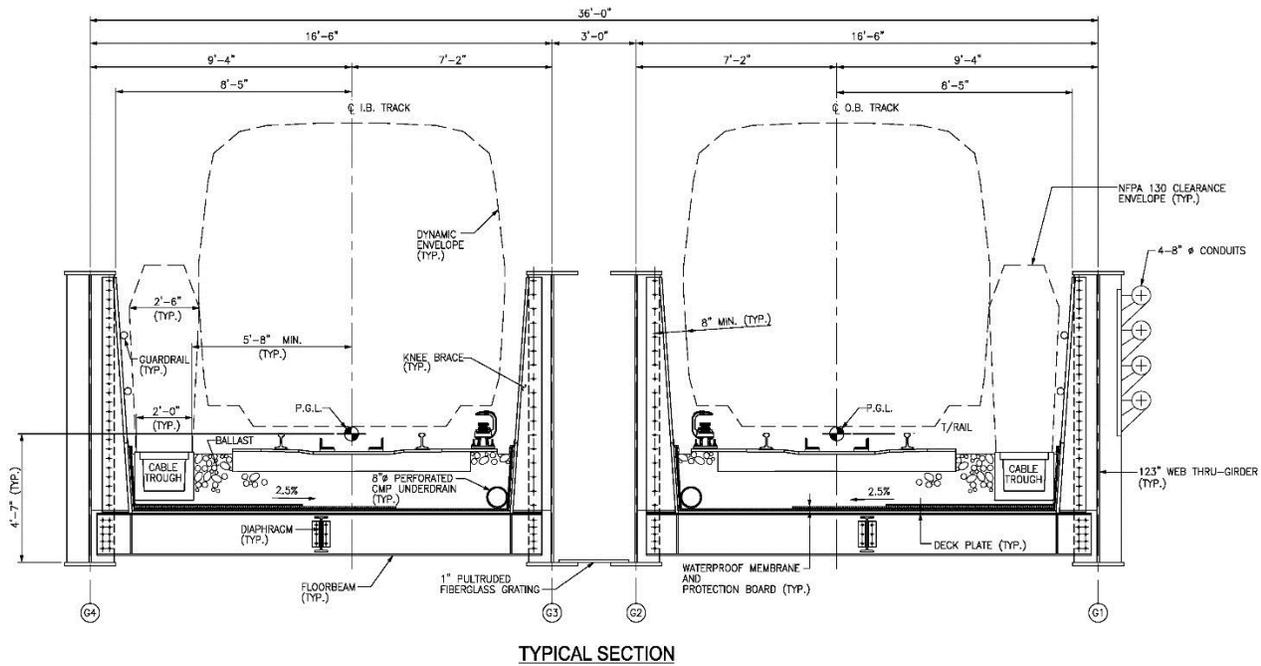
**Figure 6:** Typical section of Centreville Road Bridge
