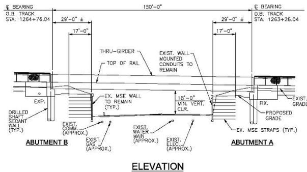
**Figure 5:** Centreville Road Bridge final design span configuration.
