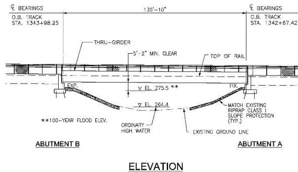
**Figure 8:** Horsepen Run Bridge span configuration.
