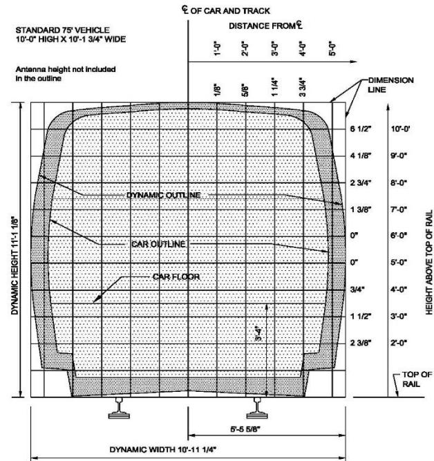
**Figure 2: Vehicle Dynamic Envelope (WMATA Design Criteria)**
