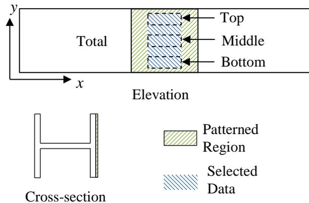
**Figure 6 Sketch of a monitored truss member, indicating the patterned and selected data area.**
