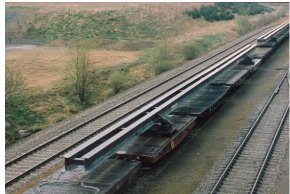
Figure 14: Exceptional rail transport of 54.16m already coupled in the workshop, Railway Bridge at Boulevard Ney a Paris, 2000, France
