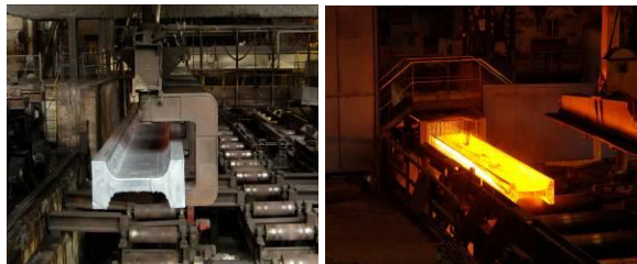
Figure 10: Rolling of structural shapes out of Beam Blanks
