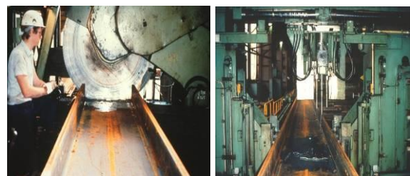
Figure 12: Cutting to exact length by saw blade, automatic drilling in the web and in the flanges
