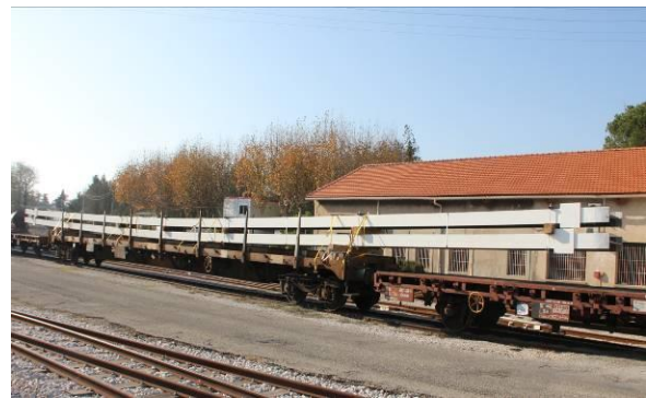
Figure 15: Exceptional rail transport of 39.7m beams with curvature about weak axis with a radius of 354m, Roadway Bridge RD257 in Arles, 2014, France
