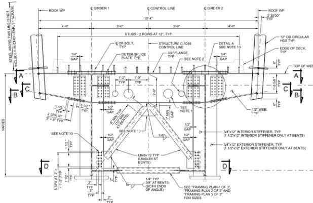
**Figure 2:** Typical cross-section of bridge
