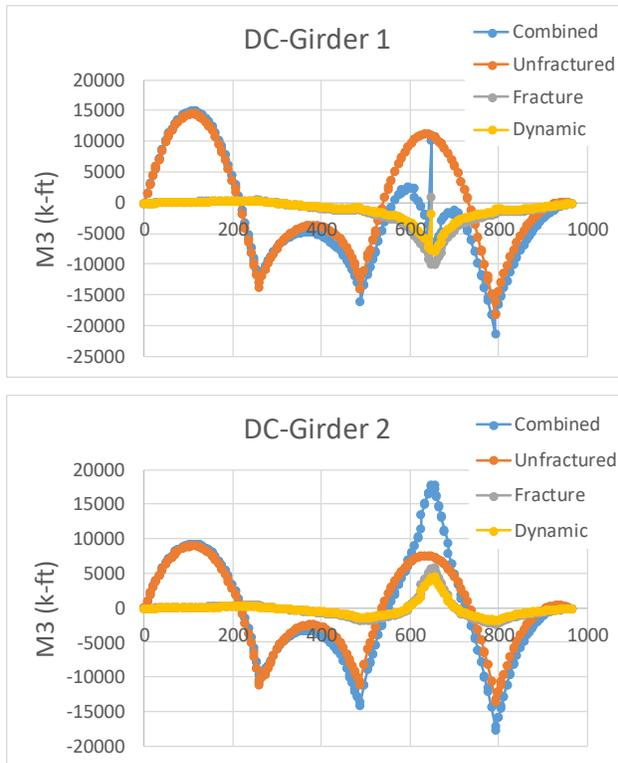
**Figure 4:** Dead Load Moment Diagrams for Girders Before and After Fracture.
