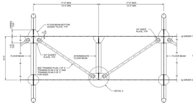
**Figure 1:** Typical Bay of Lateral Bracing
