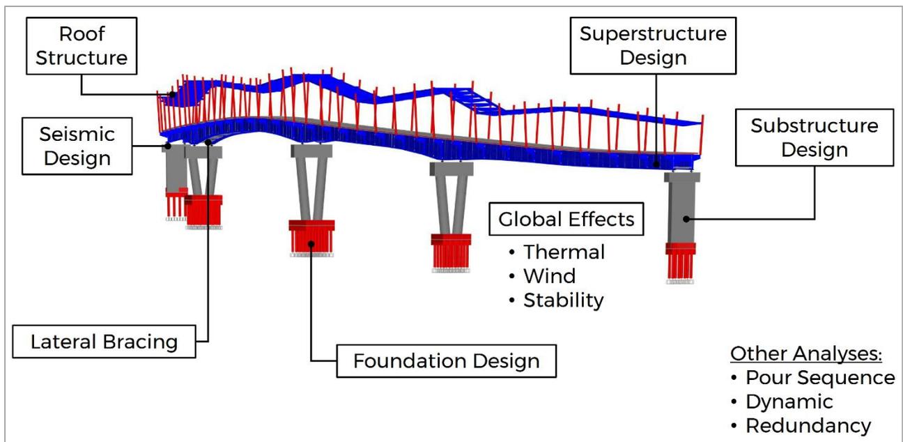
floorbeams, lateral bracing, roof beams and columns, pier caps and columns, and piles, were
