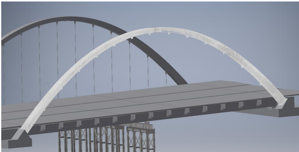
Figure 13: Lidar Arch Scans Placed in the Integrated 3D Model to Evaluate the Fabricated Shape
