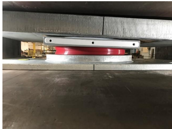
Figure 8: Disk Bearing Loaded and Rotated in a test frame.
