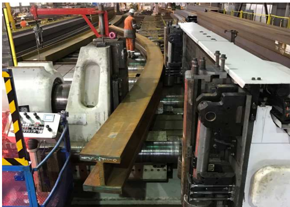
Figure 10: Curving of heavy structural sections.
