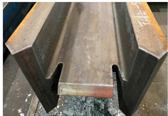
Figure 17: Detail of the weld bevel preparation.
