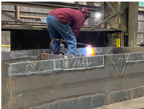
Figure 2: Heat Curving Process.
