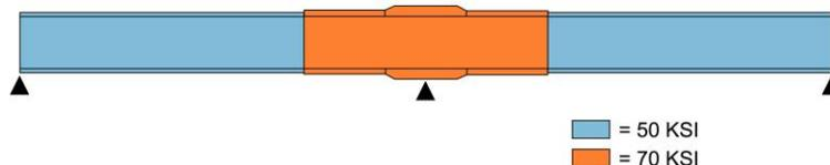
**Figure 8 Diagram of a mixed steel I-girder**
