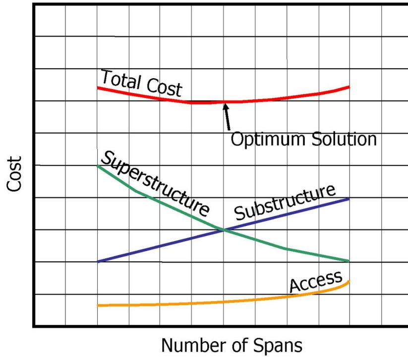
**Figure 1** Graph showing typical bridge cost curves
