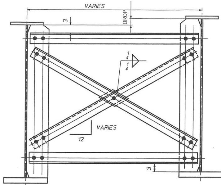
**Figure 5 Detail sketch of a typical Knocked-Down cross-frame**
