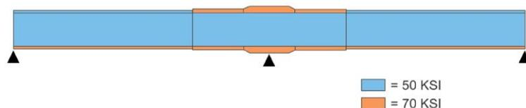
**Figure 9 Diagram of a hybrid steel I-girder**
