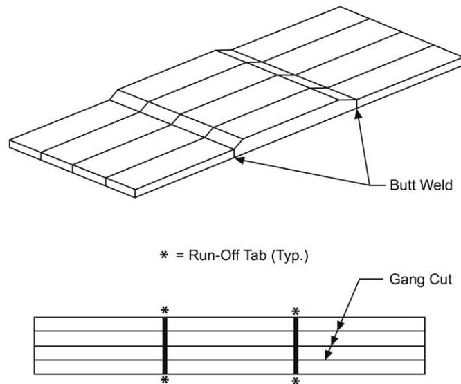
**Figure 6 Sketches showing the slabbing and stripping process**
