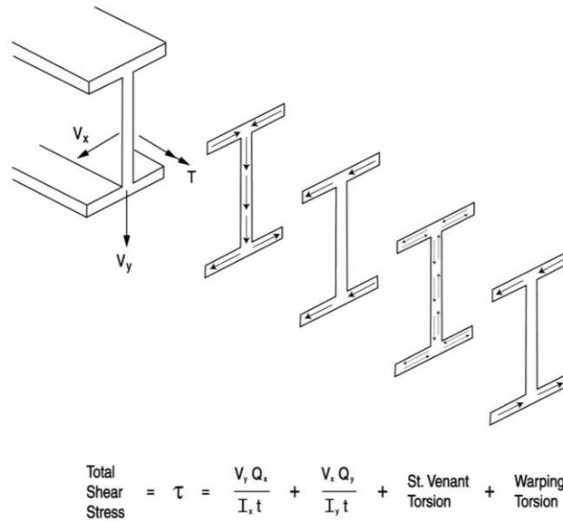
**Figure 5 Shear stresses in a curved or skewed I-shaped girder.**
