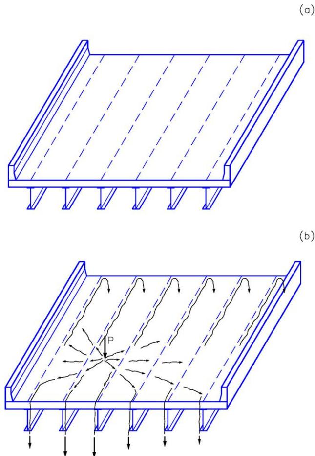
**Figure 1 Illustration of live load distribution**
