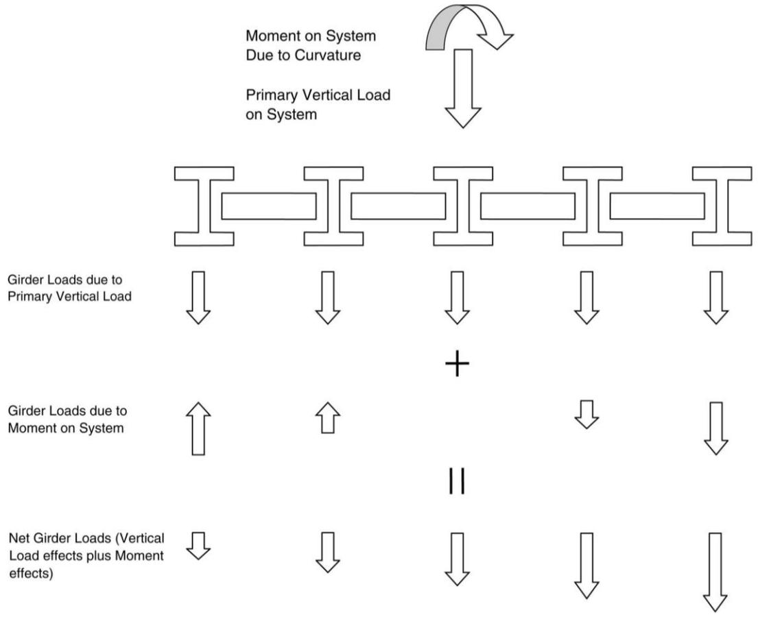
**Figure 12 Load shifting in curved girder bridge systems.**
