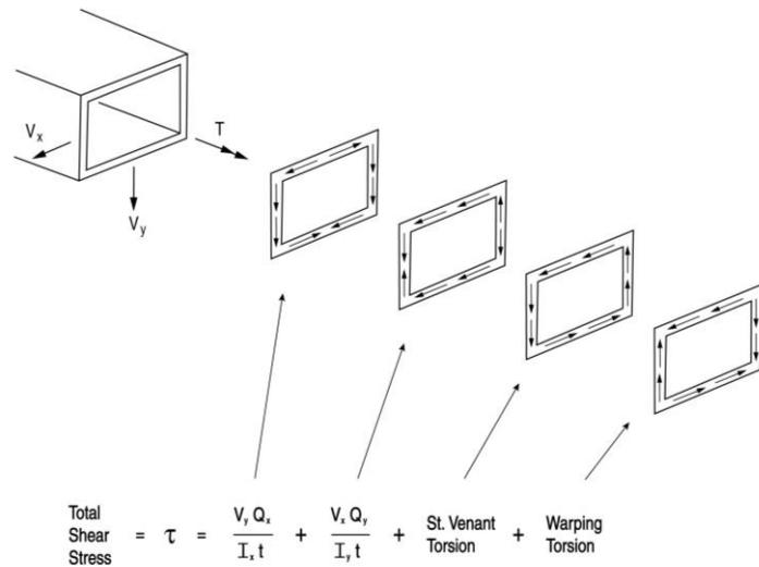
**Figure 6 Shear stresses in a curved or skewed box-shaped girder.**
