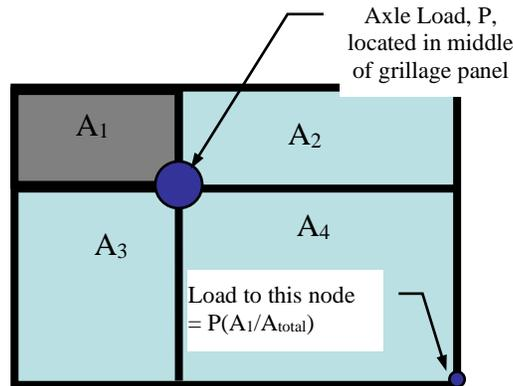
**Figure 20 Illustration of the distribution of a wheel load to various nodes in a grid analysis using area coordinate interpolation.**
