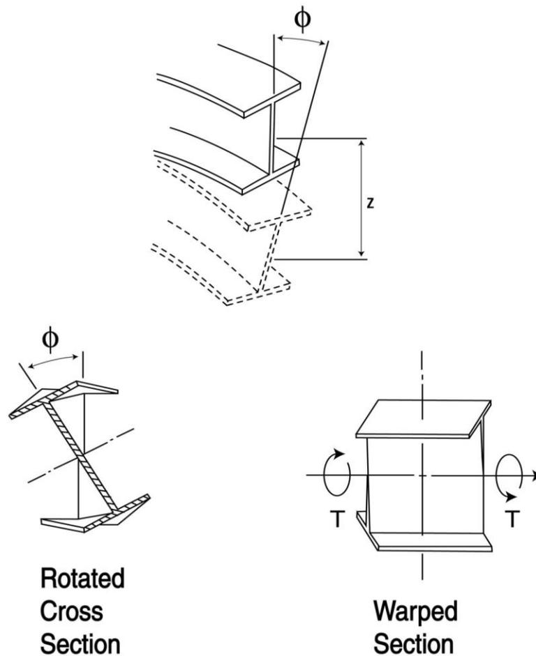
**Figure 11 Vertical deflection, twisting deformation, and warping deformation in curved I-shaped girders.**
