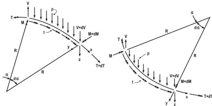
**Figure 14 Basic free-body diagrams of the M/R method [30].**
