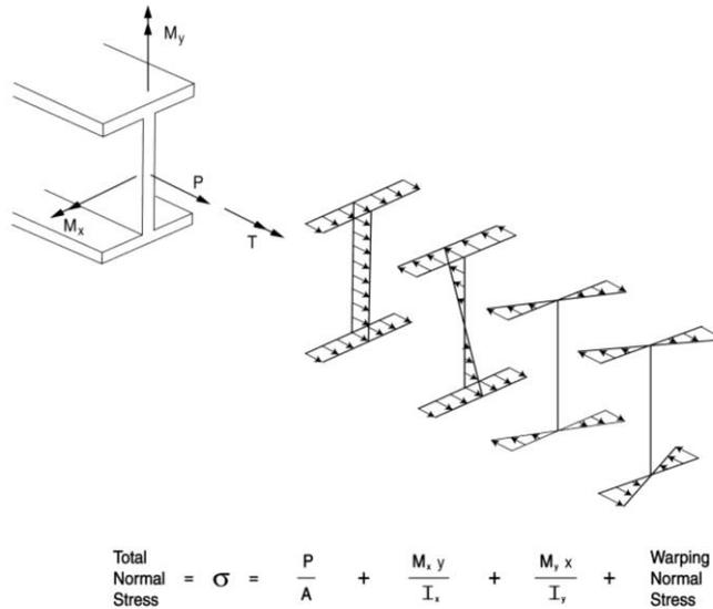
**Figure 4 Normal stresses in a curved or skewed I-shaped girder.**
