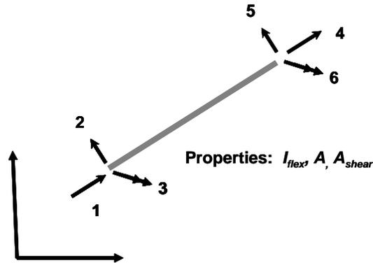
**Figure 16 Plane Frame Element.**
