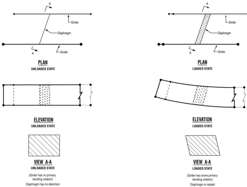
**Figure 9 System deformation of girders and cross-frames skewed to match the bridge skew.**
