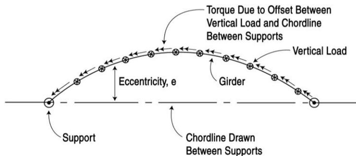
**Figure 3 Plan view of the development of torque in a curved girder**
