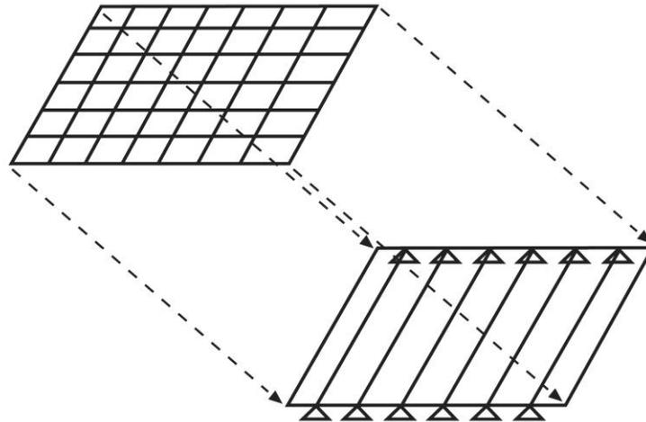
**Figure 18 A slab-on-girder bridge with a possible grillage mesh.**
