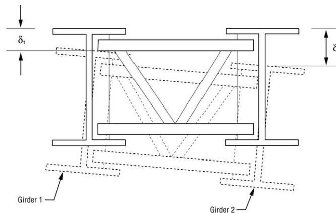
**Figure 8 System deformation of girders and non-skewed cross-frames in a skewed bridge.**
