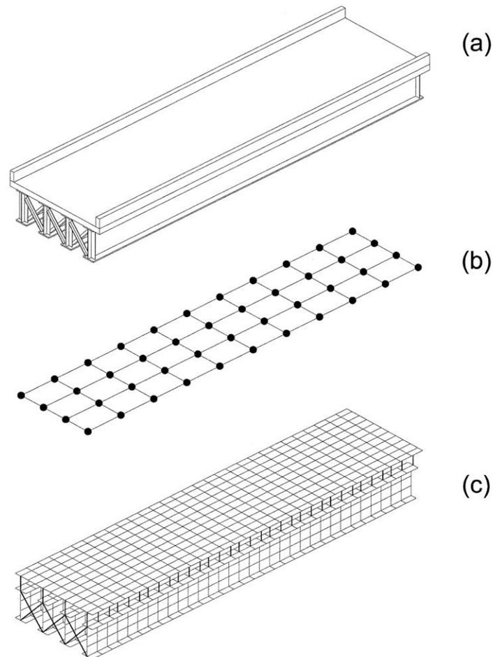
**Figure 15 Rigorous analysis method models. (a) Actual bridge, (b) 2-D analysis model, (c) 3-D analysis model.**
