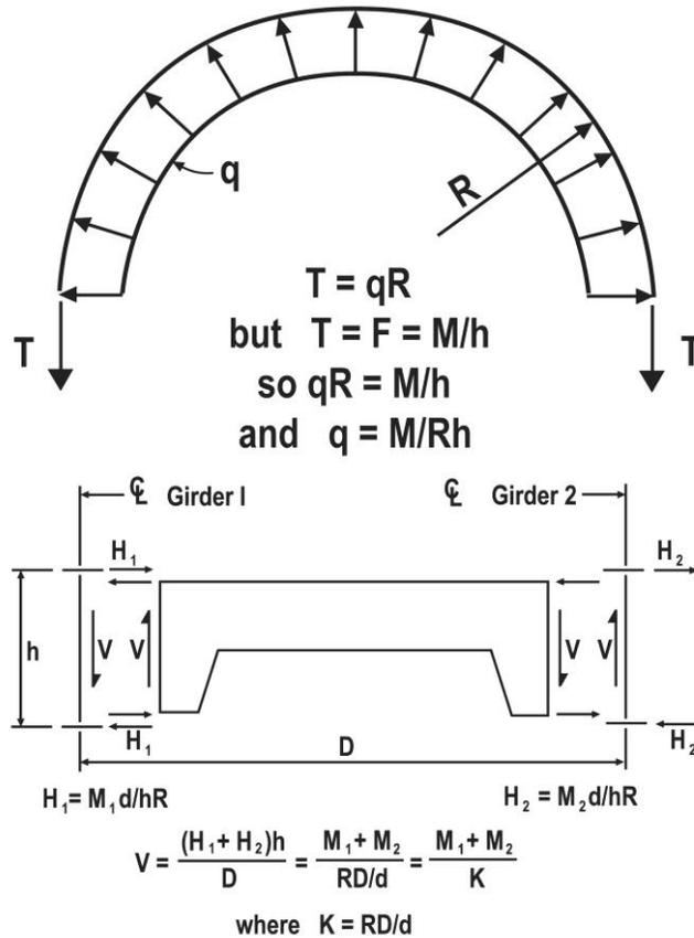
**Figure 13 Basic free-body diagrams of the V-Load method [6] (shown in a positive moment region)**
