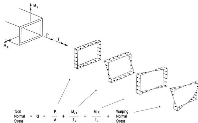
**Figure 7 Normal stresses in a curved or skewed box-shaped girder.**
