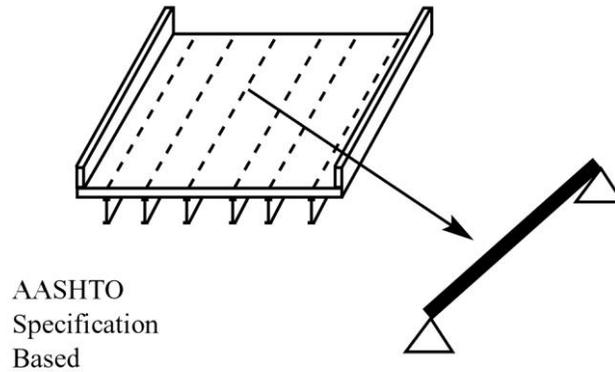
**Figure 2 Reduction in Dimensionality to a Line Girder with AASHTO Distribution Factors [31].**
