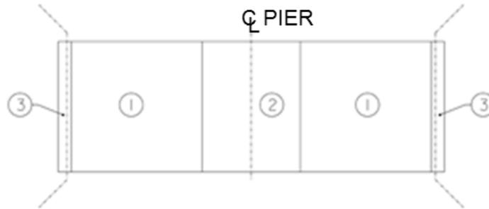
**Figure 23 Sample deck placement sequence**
