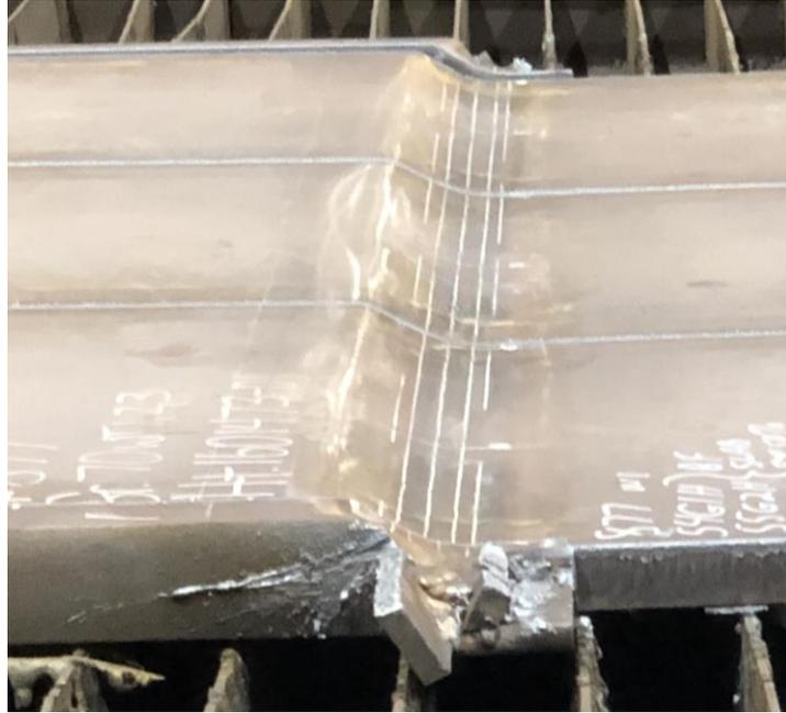
**Figure 3 Photograph of a butt-welded slab shop splice prior to cutting flanges**
