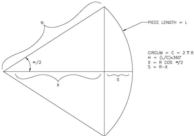
**Figure 7 Sketch of a Curved Girder Sweep**
