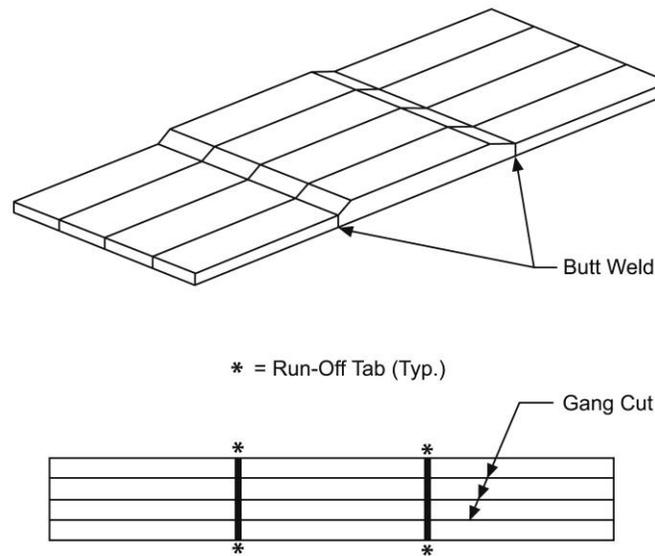
**Figure 4 Sketch Illustrating Slabbing and Stripping of Flanges**
